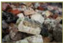
Example of the bricks found at the site. (These are from a furnace as evidenced by the molten material coating the brick.)
