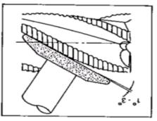
Fig.50. Angle of Wheel Inclination
