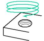
Step finishing for deep wall side milling
