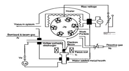
Fig.25. Physical Vapor Deposition Process
