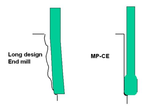
Fig.59. Comparison of MP-CE against Long design End mill
