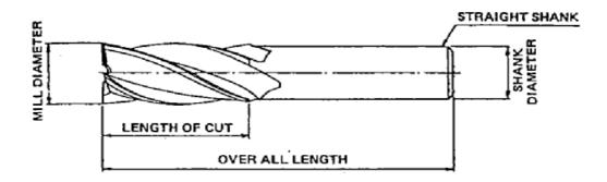
Fig.1. Straight Shank End mill
