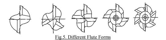
The diagram below shows the differences of 2 flutes End mill to 6 flutes End mill, where the End mill is having less flute, the chip room is bigger and better chip ejection and End mill having more flutes, it is more rigid which will have lesser deflection and breakage.
