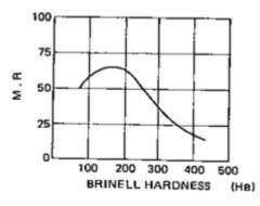
Fig.27. Relation between M.R and hardness of Steel
