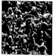
Fig.21. Micro-grain Carbide
