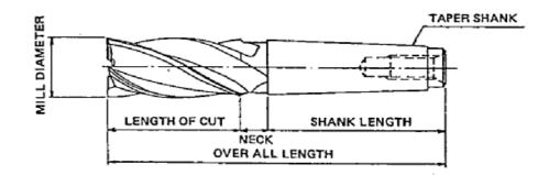
Fig.2. Taper Shank End mill
