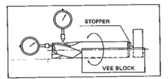
Fig.58. Measuring Cutter Run-outs
