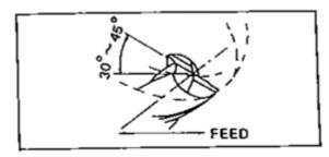
Fig.55. Re-Sharpening Gash
