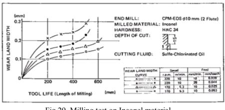
Fig.29. Milling test on Inconel material
