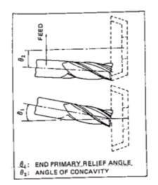
Fig.53. Grinding of End Primary Relief
