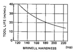
Fig.28. Relation between Tool life and Work hardness
