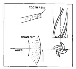
Fig.42. Position of wheel, End mill and tooth rest
