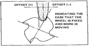
Fig.51. Adjustment of Offset
