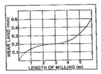
Fig.34. Relation between Wear Land & Length of Milling
