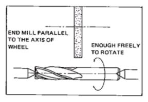
Fig.38. Holding End mill
