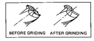
Fig.54. Comparison of before & after Gash grinding
