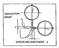
Fig.57. Checking Cutting Angle
