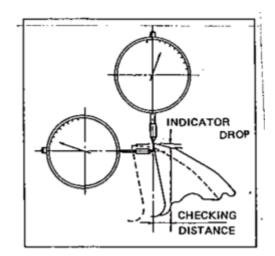
Fig. 56. Indicator Set-Up for checking Radial Relief
