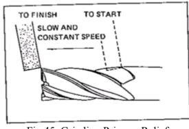
Fig.45. Grinding Primary Relief
