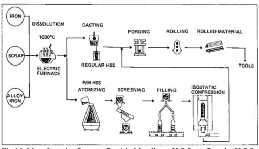
Fig.16. Manufacturing Process: Particle Metallurgy H.S.S. vs. Regular H.S.S.
