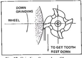
Fig.47. Grinding Secondary Clearance
