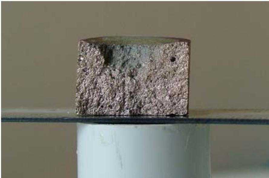
**Figure 7.9: Photograph of an impact specimen thinly coated with gold.**
