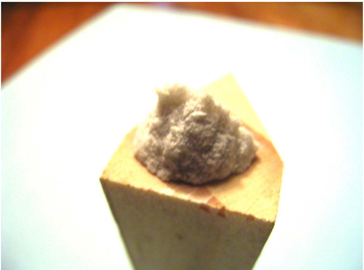
Figure 8.4: Photograph of shear cone piece, typical of all fractured impact specimens showing cleavage steps radiating around the surface of the cone. The cones are roughly 45 degrees and are a result of shear stress concentration along some diagonal plane with the composite.
