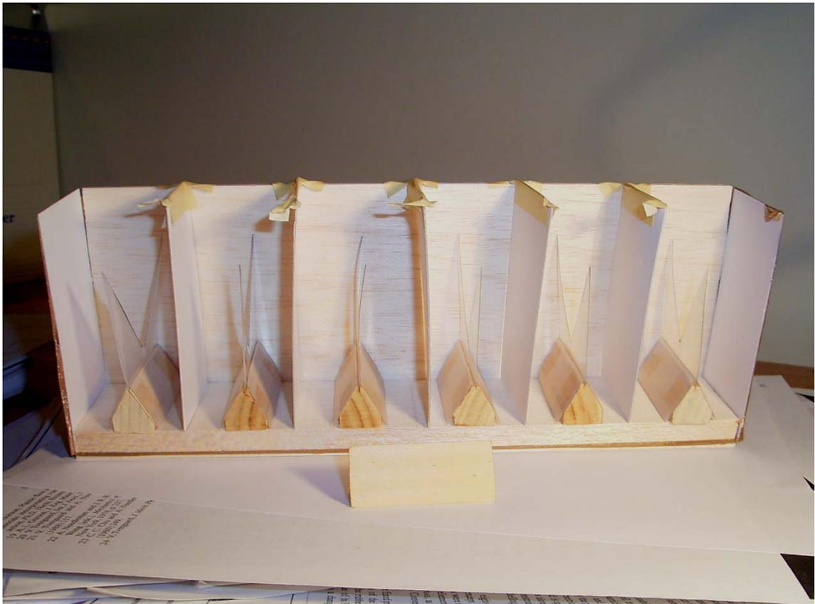
**Figure 5.6: Internal view of the short bar specimen mould showing the wooden tongue in the foreground and the transparent polypropylene chevron slots.**
