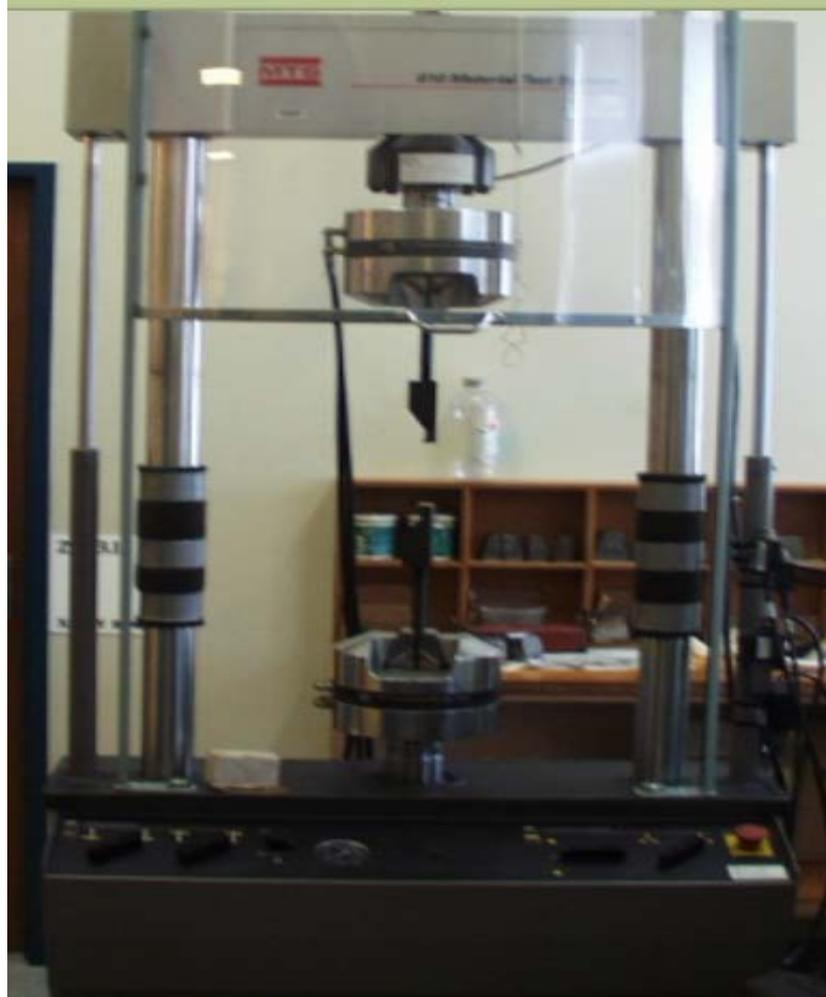
**Figure 6.1: MTS 810 Material Testing System.**
