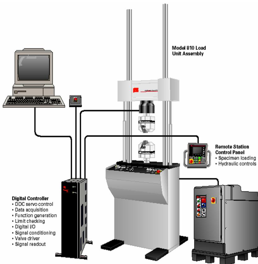
**Figure 6.3: The operating systems of MTS 810 Material Testing Systems (MTS 810 Material Testing Systems, 2003).**
