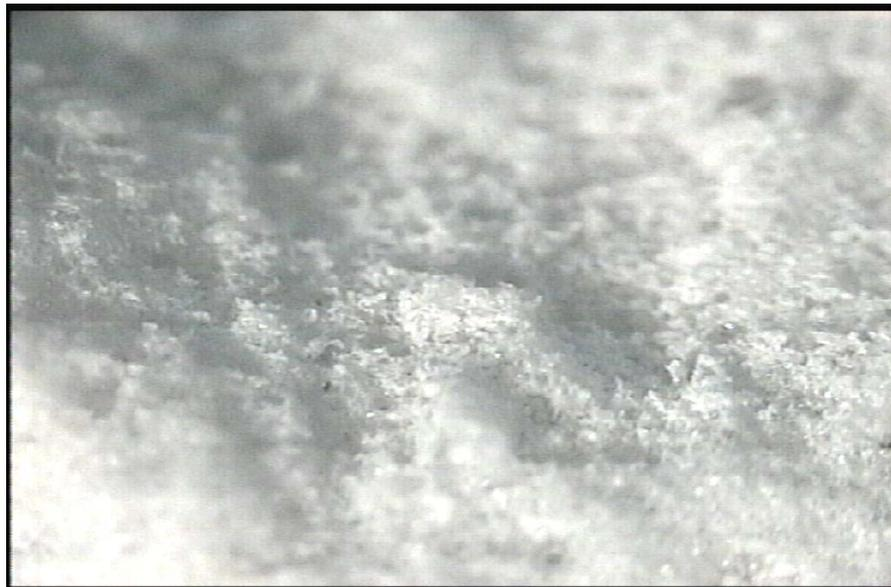
**Figure 7.3: Image captured from a stereomicroscope showing multiple cleavage steps.**
