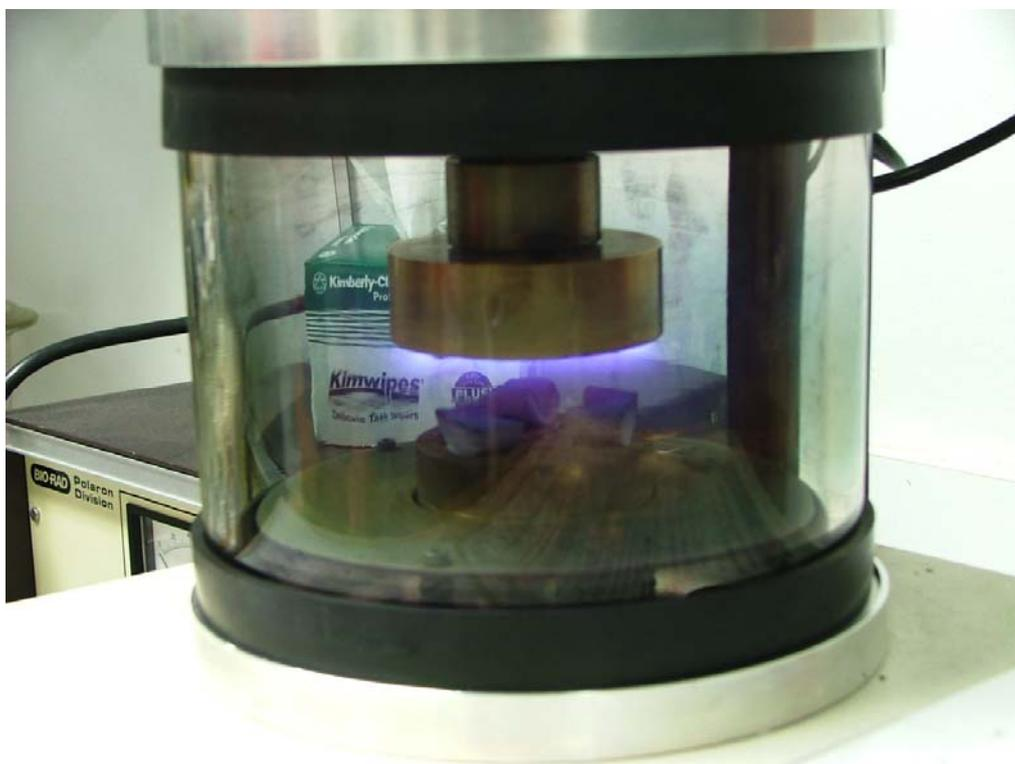
**Figure 7.8:** Argon gas molecules are ionized and are accelerated into the gold plate. Gold atoms are preferentially deposit on the sample.
