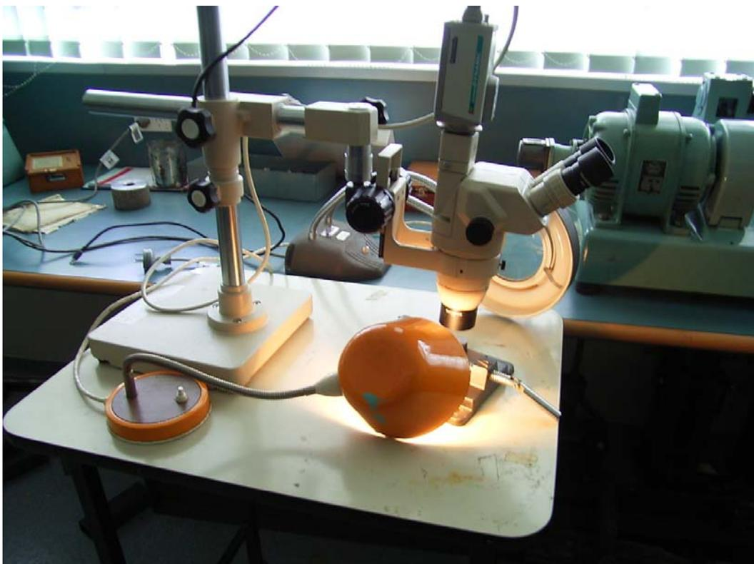
**Figure 7.2: Stereo microscope set up at USQ with lamps for illumination and a CCTV for image capture.**
