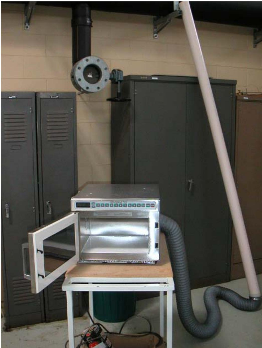
**Figure 3.5: Modified microwave and its peripherals (source: Cheng, 2003)**
