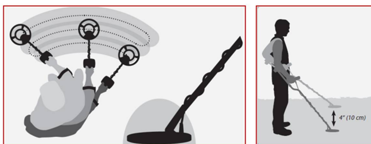
Figure 1.1: Horizontal swing cycle and elevation of an electromagnetic coil above the ground.
