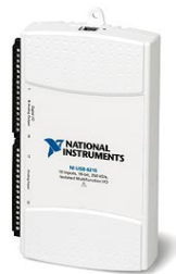
Figure 5.6: The NI USB 6210 (National Instruments Corporation n.d.) with 256kS/s sampling rate, 16 analog inputs, 4 digital inputs and 4 digital outputs.
