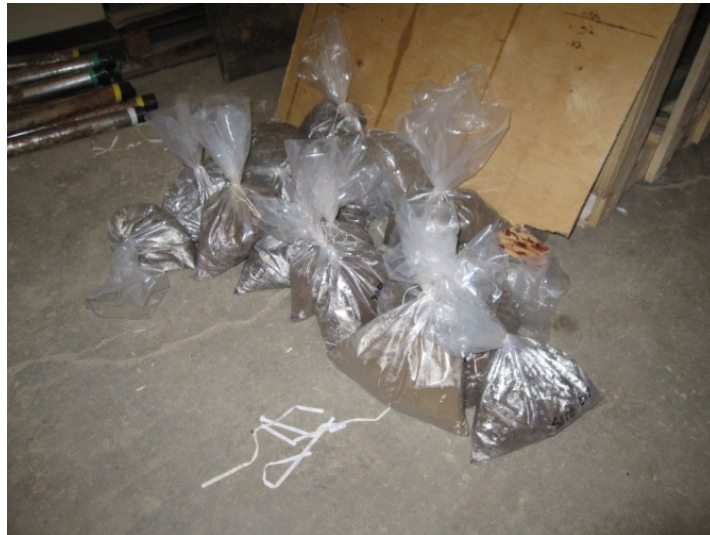
Figure 4.4 – Samples bagged and sealed prior to laboratory testing
