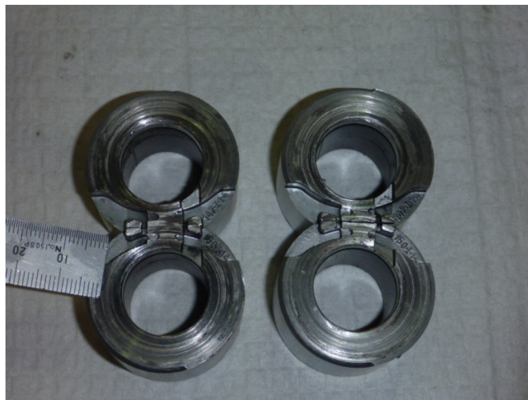
Figure 3.5: Abrasion wear on gear pump shaft bearing
