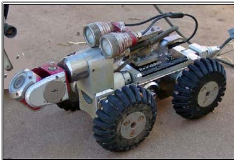
Figure 2-5 Sewer inspection tractor
