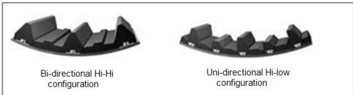
Figure 3.7: Liner and lifter configurations (Source:
