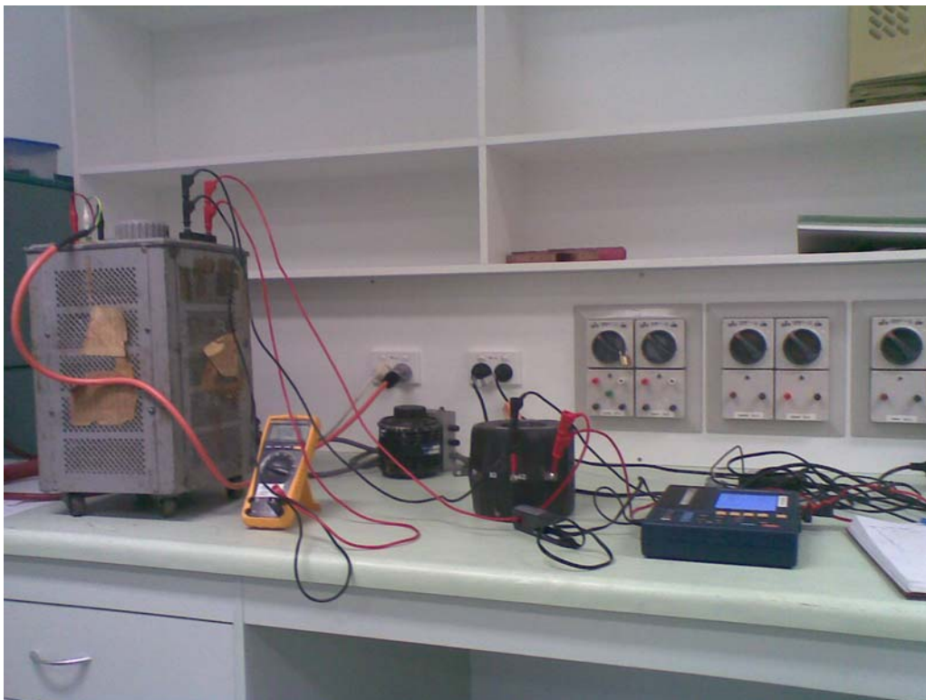
Figure 4.7 - Current Transformer Bench Testing
