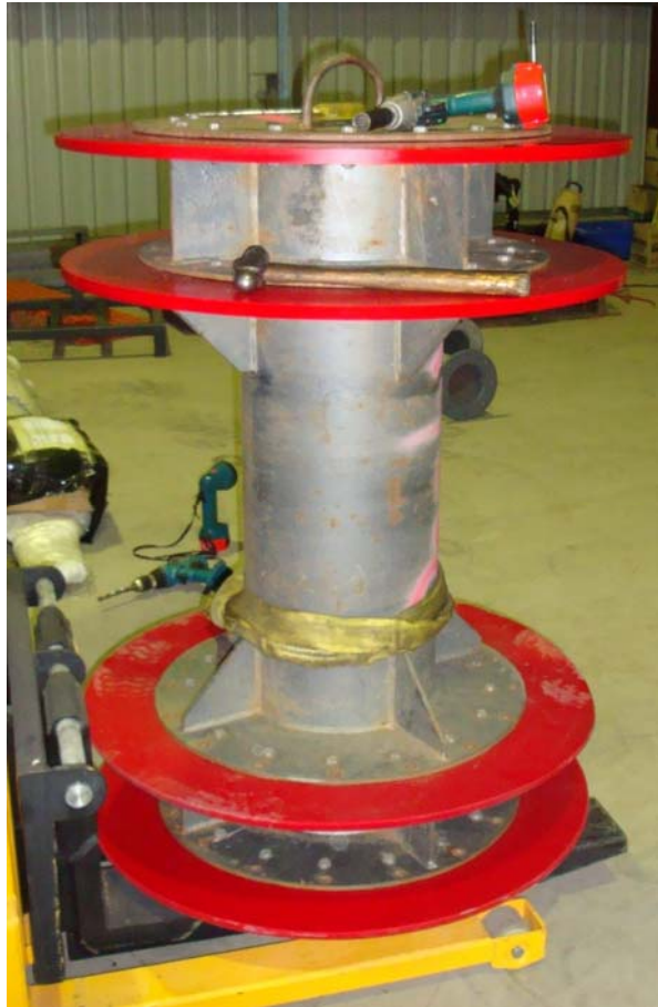
Figure 5.1 – Metal Mandrel Pig Used at Stanwell Pipeline
