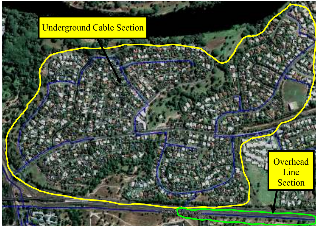
Figure 2.5 – HV Lines and Cables of Distribution Feeder ROPL-04
