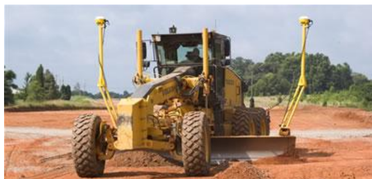
Figure 1.1: Trimble GCS900 on a Motor Grader with Dual GPS (Trimble, 2010)
