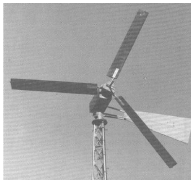
Figure 3.6: Furl control showing furling rotor (Source unknown)
