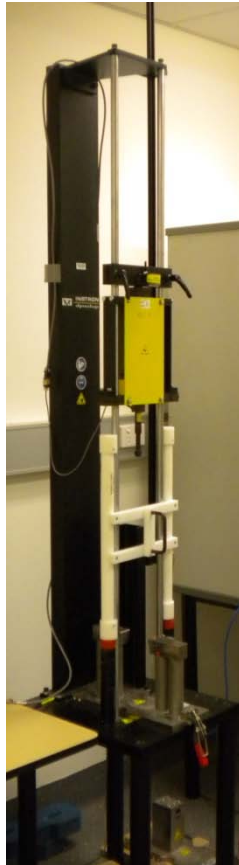
Figure 5.11. Impact Testing device.
