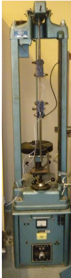
Figure 5.1. Creep Testing System
