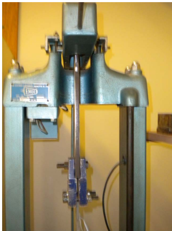
Figure 5.3. Upper Section of the Load Train Attached to Cantilever System.
