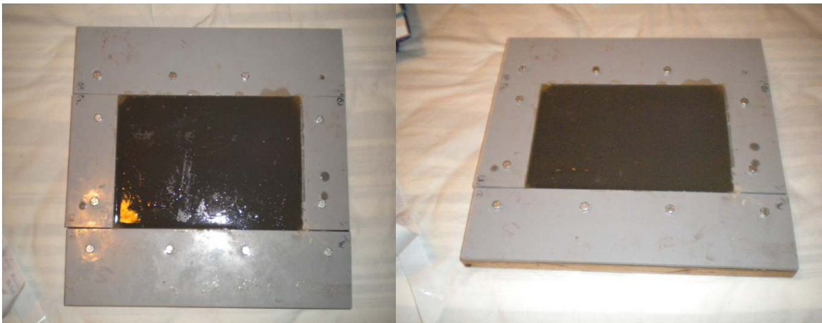
Figure 5.1. The Mould Used for Sample Preparation
