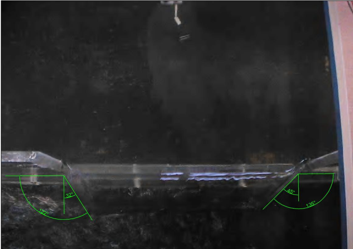
Figure 5-13 – Long Weir Angle of Discharge
