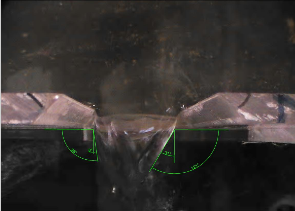
Figure 5-6 – Discrete Weir Angle of Discharge
