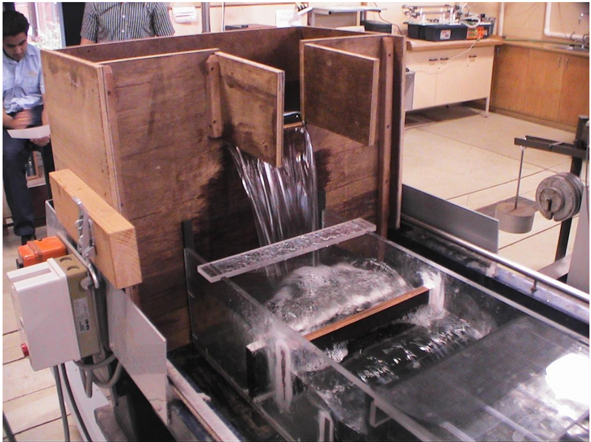
Figure 4-2 – Intake box to ensure flow is contained in narrow flume
