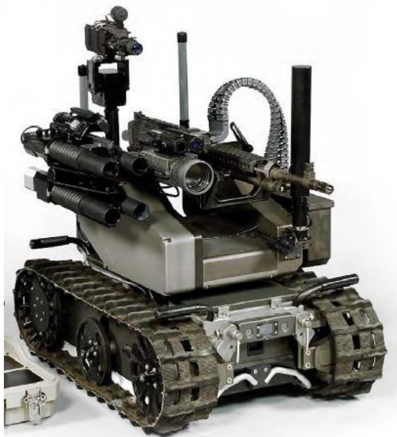
Figure 3 SWORDS robot system equipped with M240 7.76mm 100 rnd machine-gun (Defence Review, 2010)
