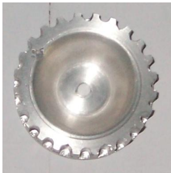
Figure 17 – Final, fully machined drive wheel component
