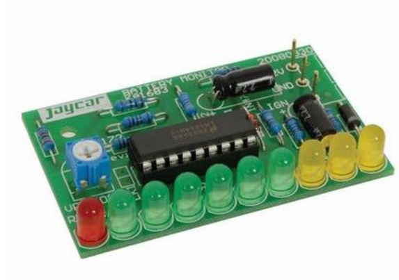
Figure 47 - Battery level monitor, Jaycar kit KA1683 constructed and ready to be implemented
