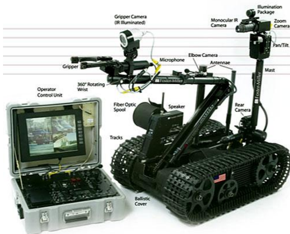
Figure 1 -TALON bomb defusal and placement robot (Robot Central, 2010)
