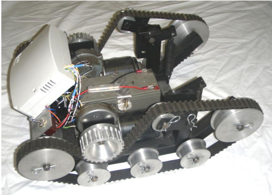
Figure 46 - Showing the placement of the battery in relation to the motors and chassis
