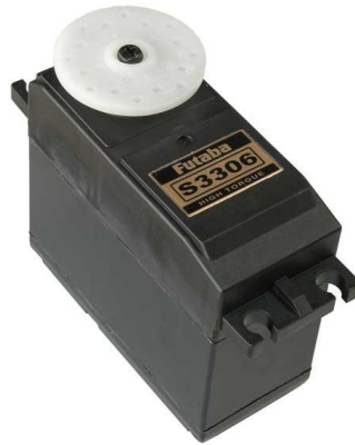
Figure 30 - Servo motor used in the camera adjustment system (Futaba - Active Robots 2010)
