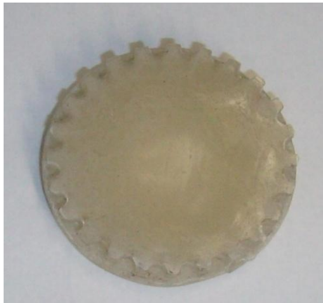
Figure 15 - Wax mould formed from solid model
