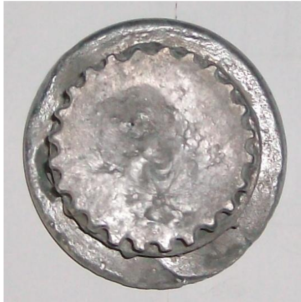
Figure 16 - Rough cast of aluminium drive wheel
