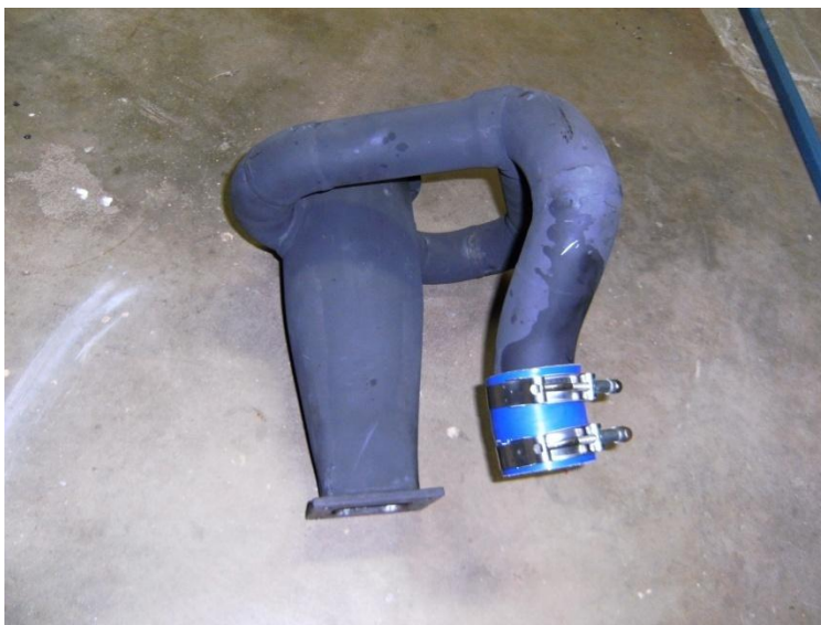
Figure 6.4: Side view of the completed combustion chamber
