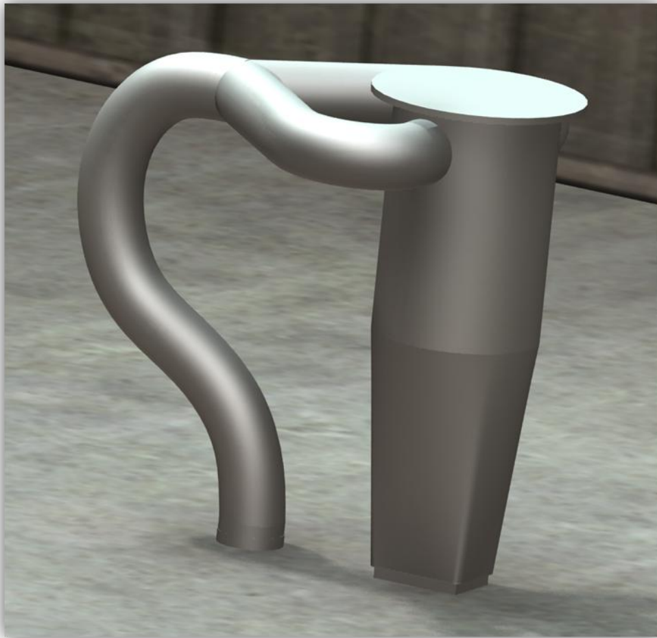
Figure 6.1: The completed pre-construction 3-D model of the combustion chamber.
