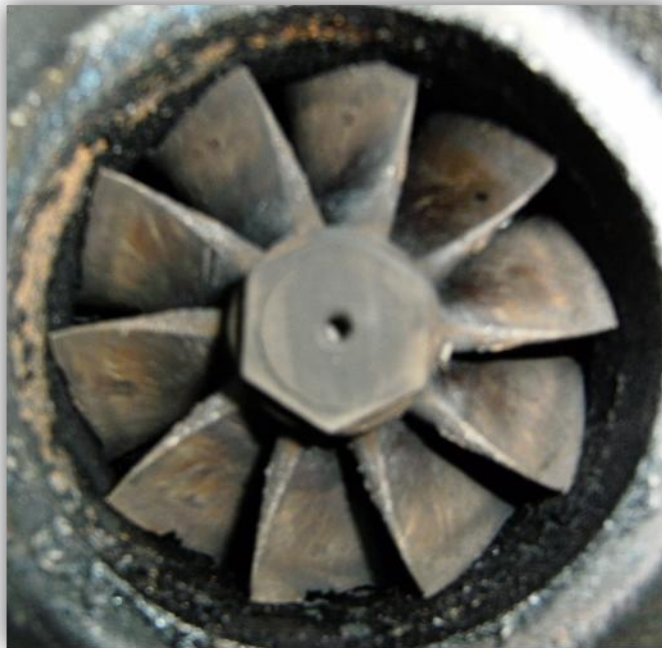
Figure 7.3: Close up of turbocharger turbine wheel post-failure (note chips on blade edges)
