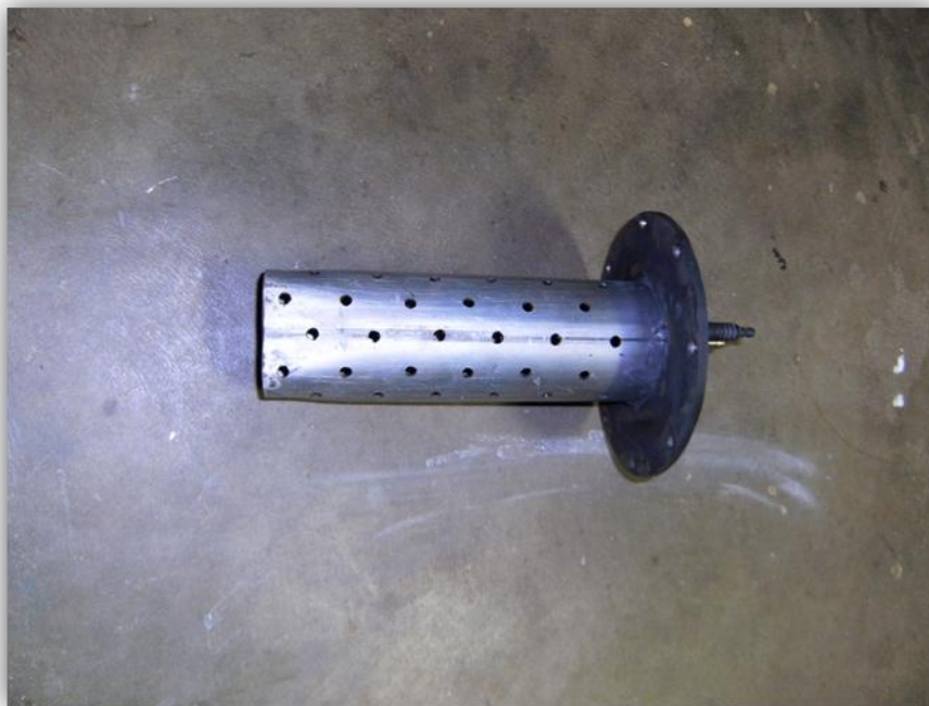
Figure 6.6: Side view of the completed combustion liner
