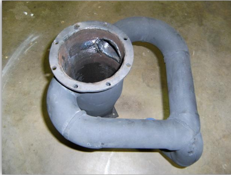
Figure 6.5: Top view of the completed combustion chamber
