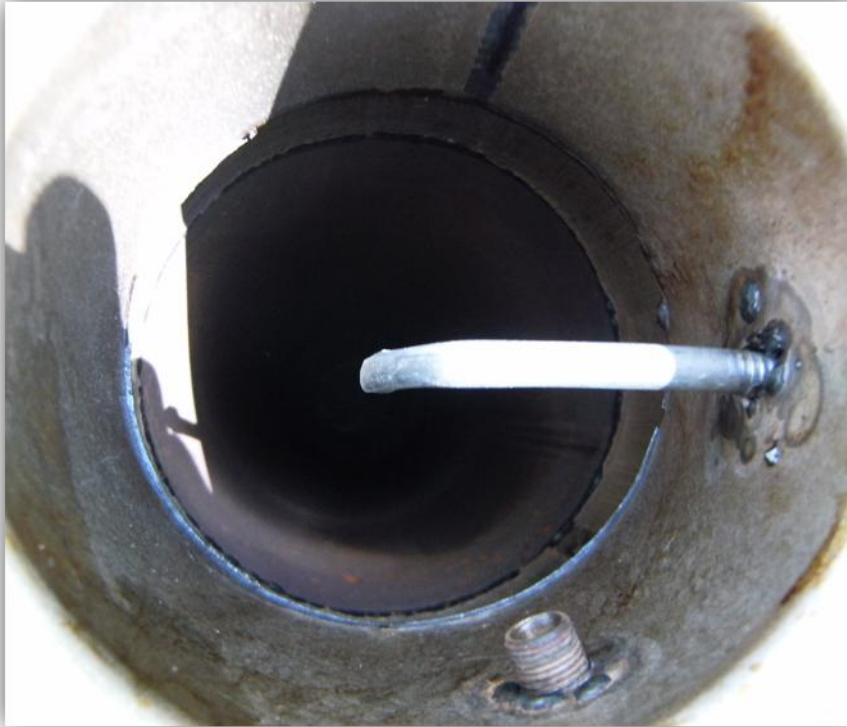
Figure 6.9: Top view of the completed afterburner showing secondary fuel injection
