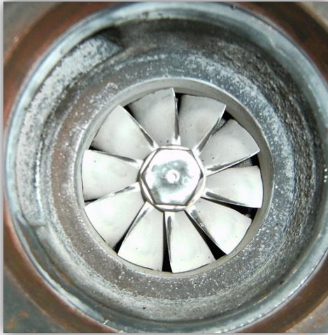
Figure 7.2: Close up of turbocharger turbine wheel pre-failure
