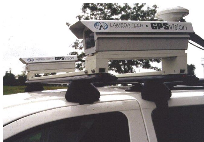
Figure 2.8: GPS, INS, and Cameras
