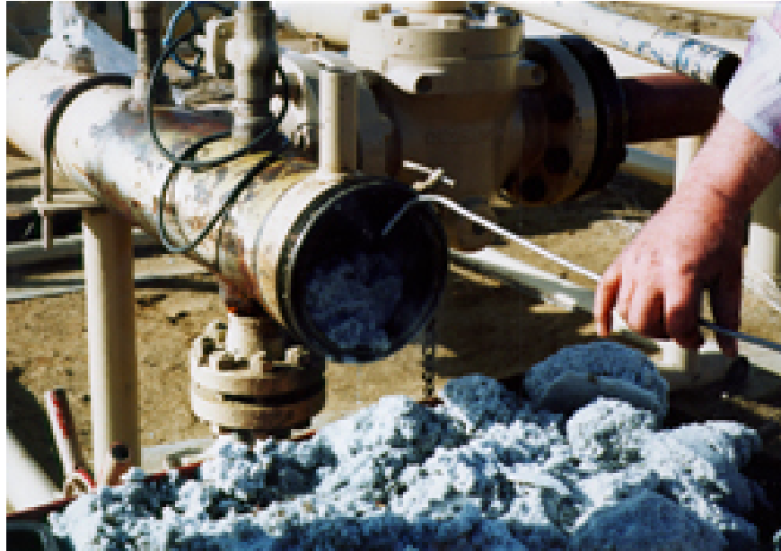
Figure 2.4: An example of a natural gas hydrate form in a gas distribution pipe. (adapted by Benton, A., 2010)
