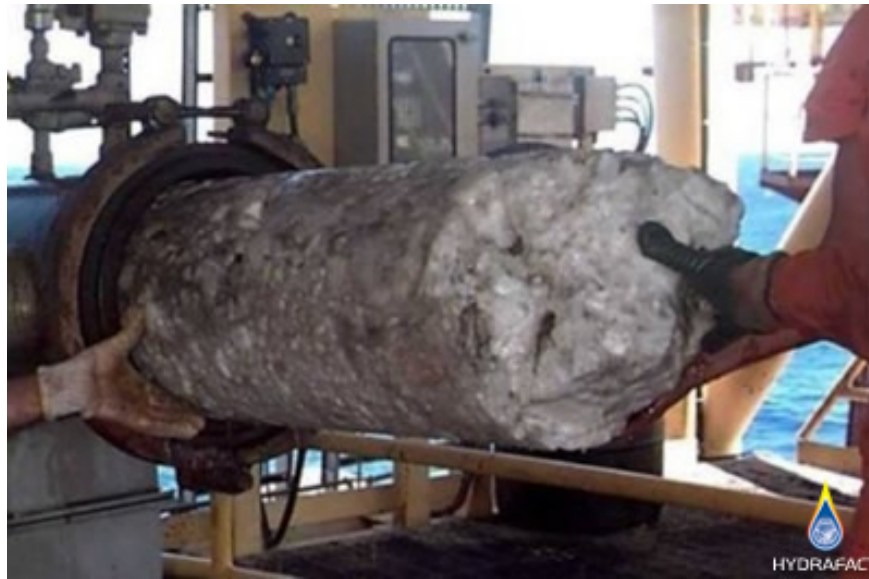
Figure 2.3: An example of a natural gas hydrate plug. (adapted by Harriot Watt Institute of Petroleum Engineering)
