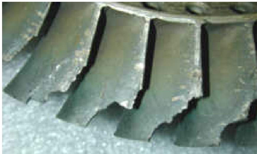
Figure 2.2: Turbine blade embrittlement caused by over firing. (adapted by Accident and Failure Analysis Consultants)
