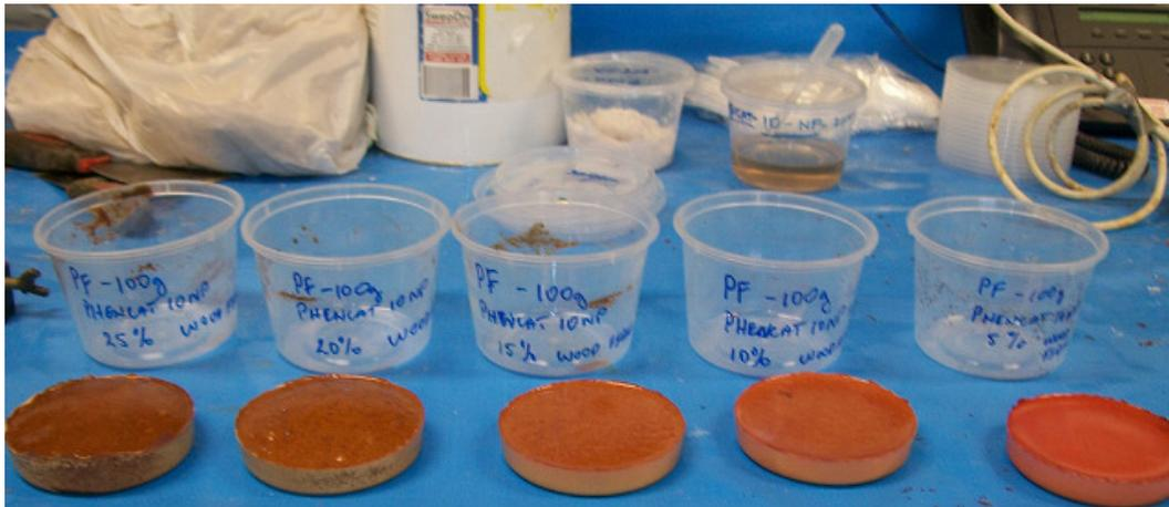
Figure 21: Phenolic resin samples with the different volumes of wood fibre
