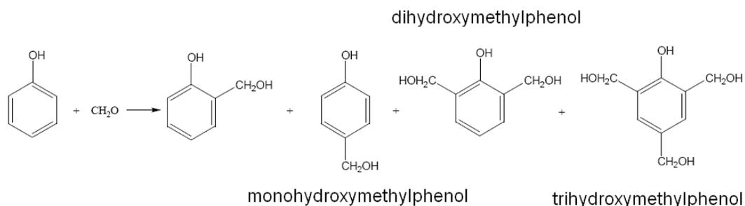
**Figure 8: Reaction of phenol with formaldehyde (Adapted from Tyberg 2000, p.4)**
