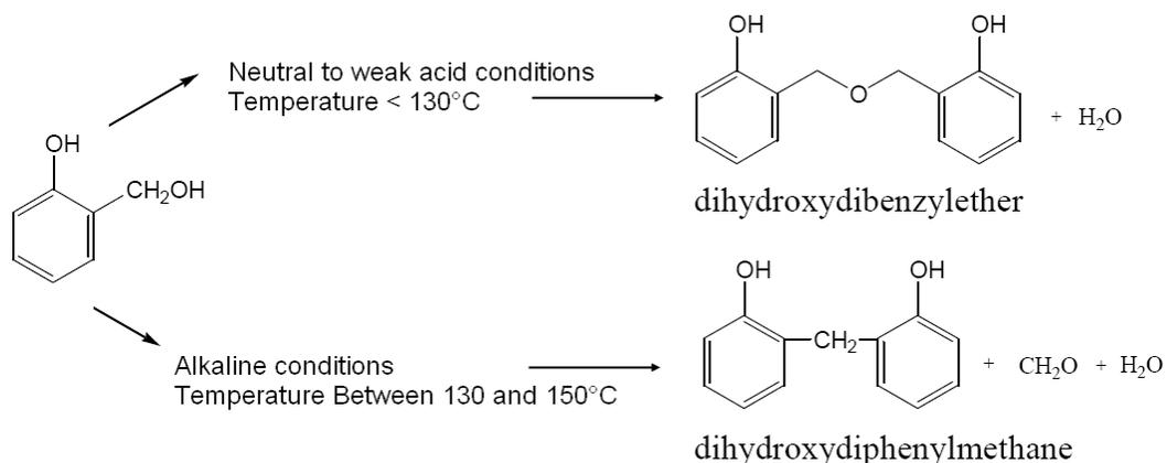
**Figure 9: Resol prepolymer formation (Adapted from Tyberg 2000, p.4)**
