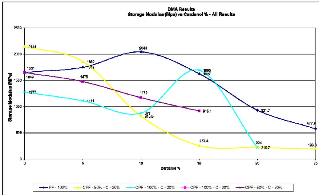
Figure 41: Graph of all DMA Storage Modulus (MPa) results for all resin types
