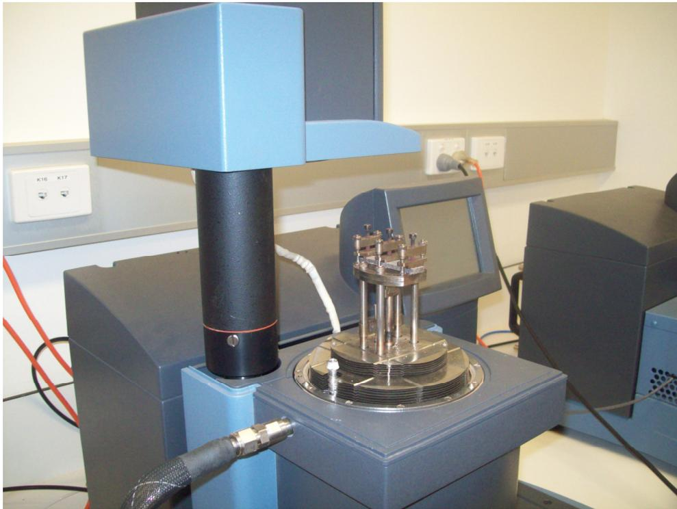
Figure 19: DMA test machine with sample for testing
