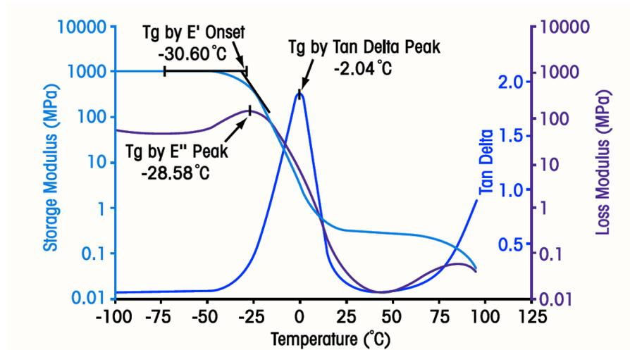
Figure 18: An example of the attributes measurable using DMA testing
