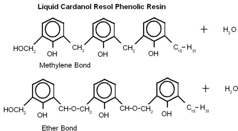
Figure 11: Bonded Liquid Cardanol Resole Phenolic Resin (Cardona 2009)
