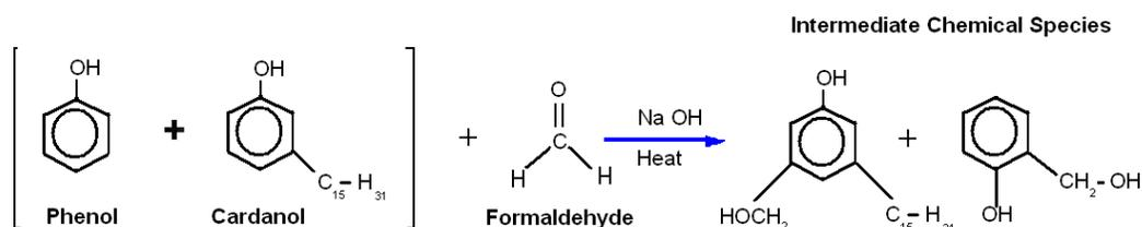
Figure 10: Phenol and Cardanol Bonding to create CPF resin (Cardona 2009)
