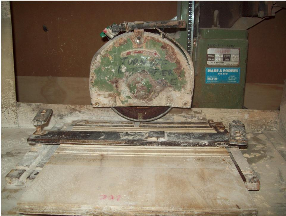
Figure 134: Hafco Tile cutting machine used for cutting of samples
