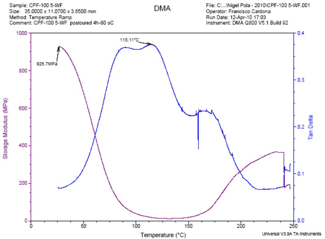
**Figure 121: CPF 100% resin - (Cardanol 20% of CPF) Wood fibre 5%**
