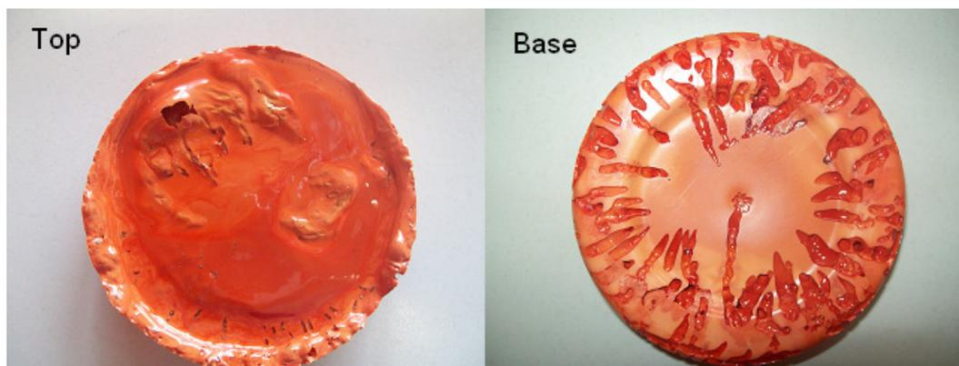
**Figure 23: PF resin sample produced during study showing excessive voids from excess catalyst in reaction.**
