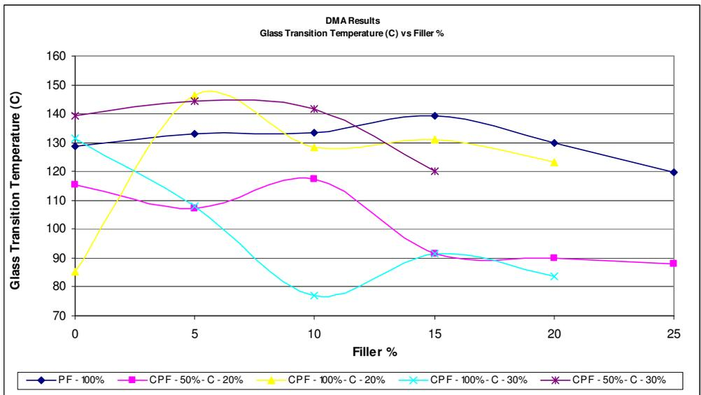
Figure 45: DMA Glass Transition Temperature (Tg) results for all resin types
