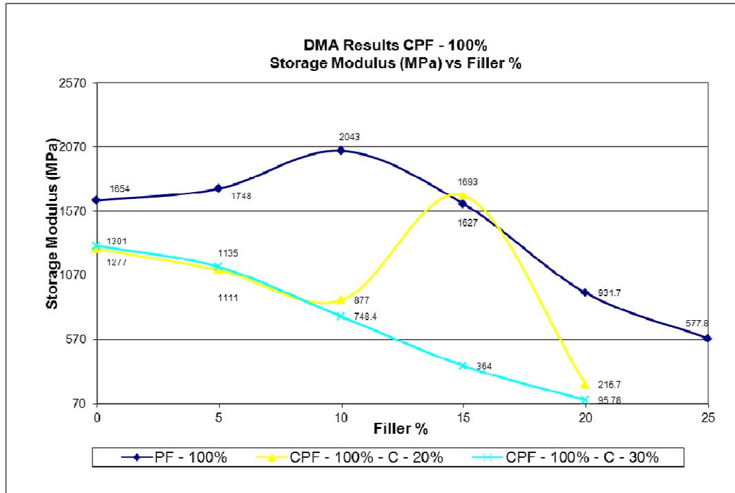
Figure 100: Graph of DMA – Storage Modulus vs. Filler % All CPF 100% comparison with PF resin
