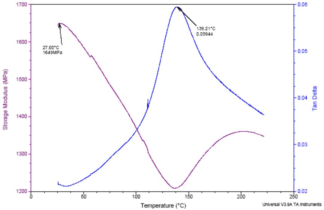
Figure 130: PF 50% CPF 50% resin - (Cardanol 30% of CPF) Wood fibre 0%
