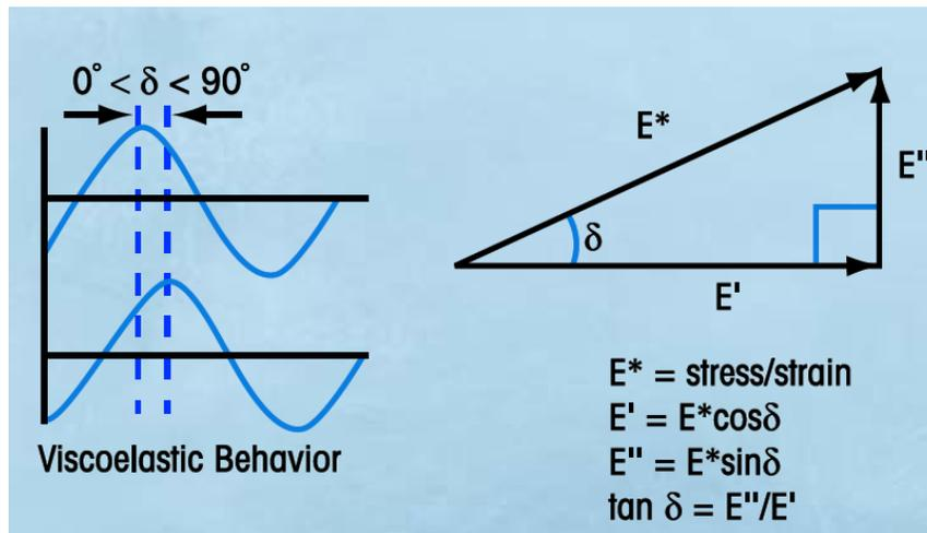
Figure 17: Dynamic Oscillatory test details (TA Instruments 2008)
