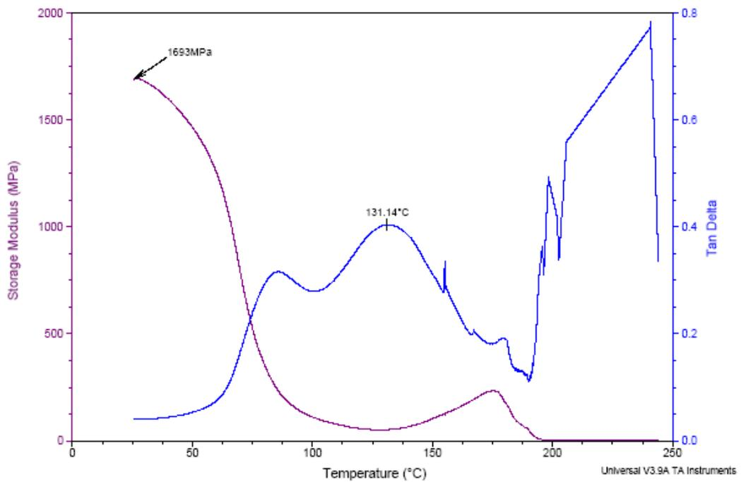
Figure 123: CPF 100% resin - (Cardanol 20% of CPF) Wood fibre 15%
