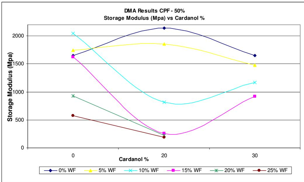
Figure 43: Graph of DMA results of Storage modulus vs Cardanol% - CPF 50%
