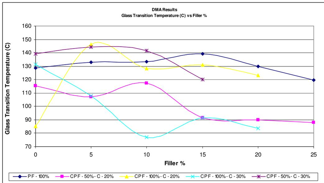
Figure 88: Graph of DMA Glass Transition Temperature vs Filler % All Results
