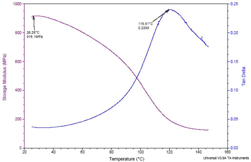
Figure 133: PF 50% CPF 50% resin - (Cardanol 30% of CPF) Wood fibre 15%
