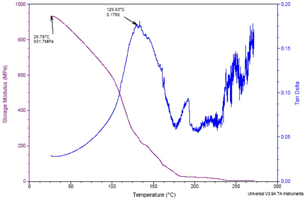
Figure 113: 100% PF resin - Wood fibre 20%
