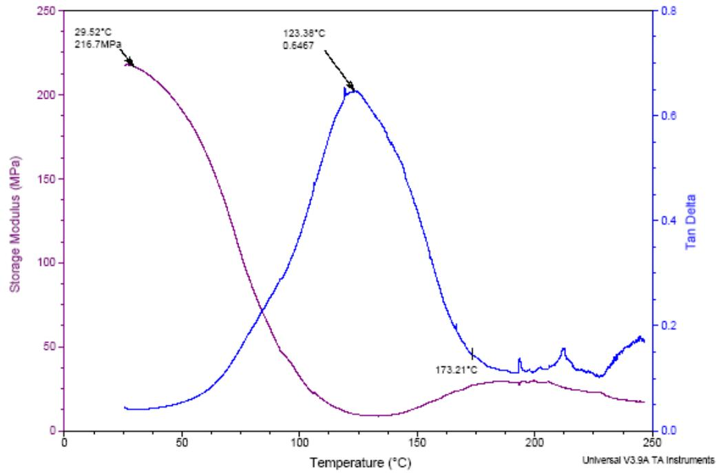
Figure 124: CPF 100% resin - (Cardanol 20% of CPF) Wood fibre 20%
