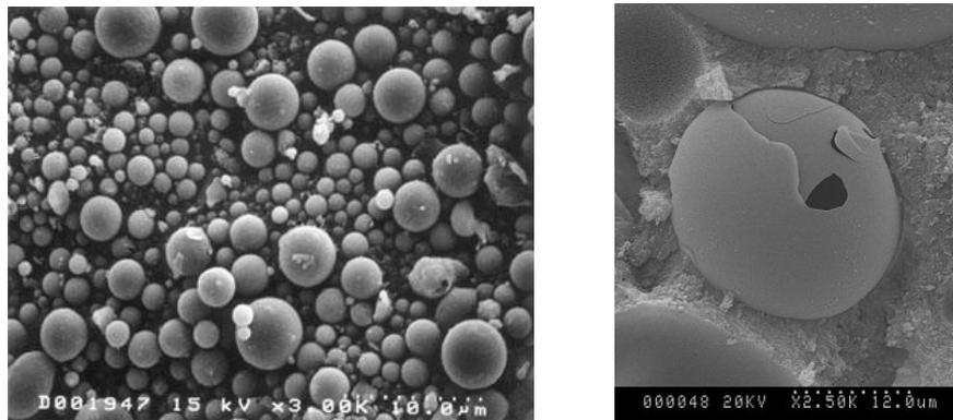
**Figure 16: Fly ash particles LHS (US department of Transportation 2006) and glass microspheres RHS (concrete canoe 2010)**
