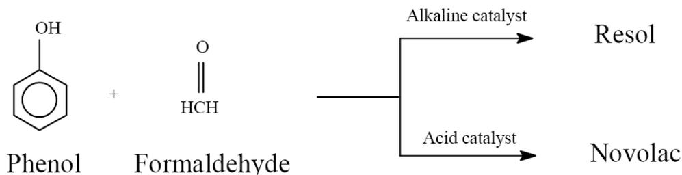
Figure 7: Synthesis pathway of Resol and Novolac (Adapted from Painter and Coleman 2000, p.1).
