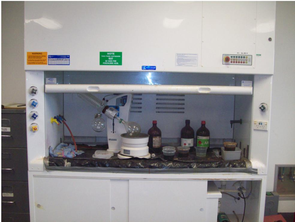
Figure 136: Fume cabinet holding oil bath for bonding Phenol and Cardanol
