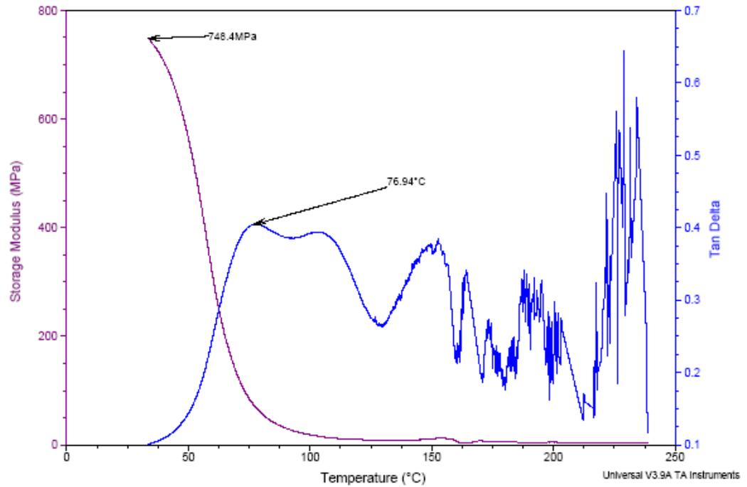
Figure 127: CPF 100% resin - (Cardanol 30% of CPF) Wood fibre 10%
