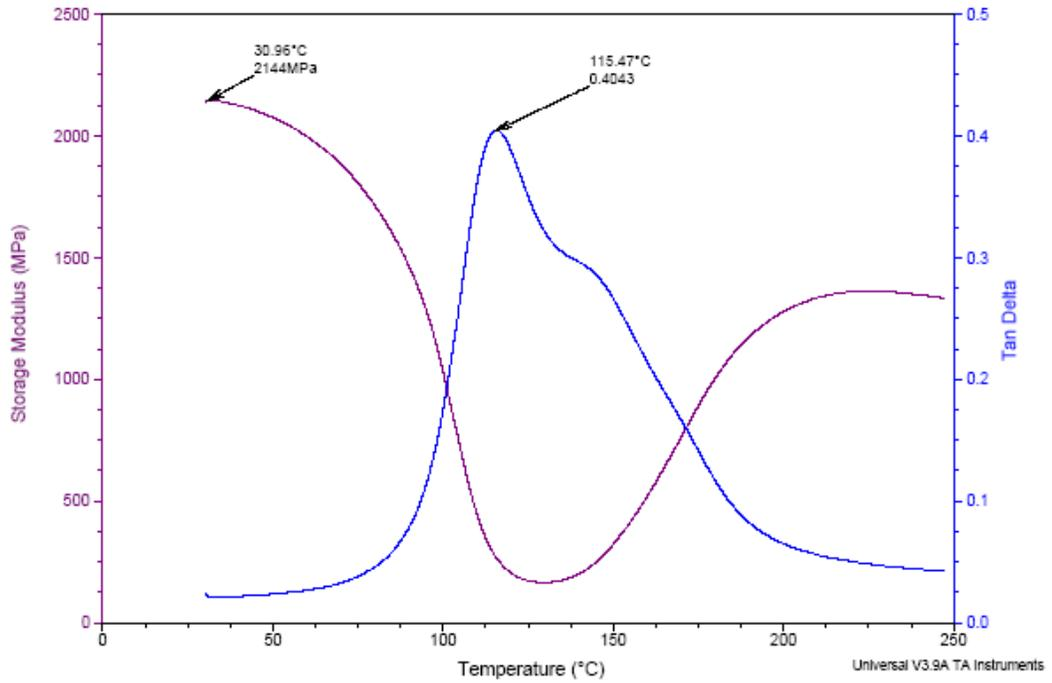
Figure 115: PF 50% CPF 50% resin - (Cardanol 20% of CPF) Wood fibre 0%
