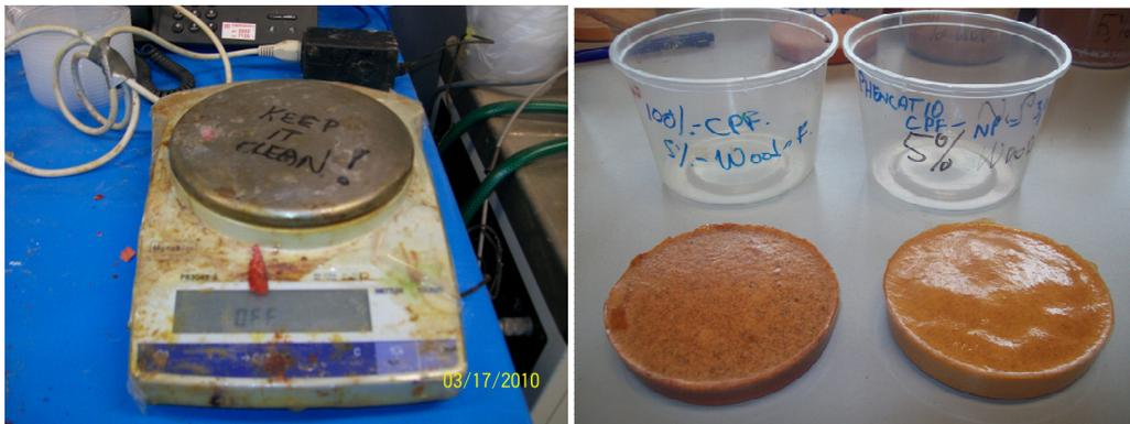
Figure 137: Measuring Scales (LHS) and Flexural Test moulds (RHS)
