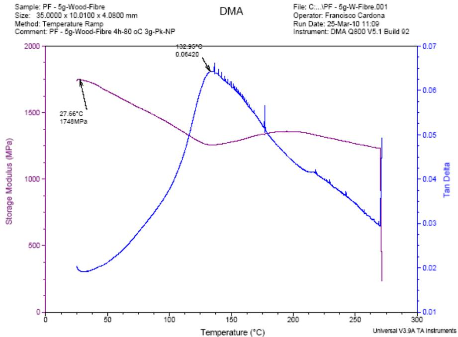
Figure 110: 100% PF resin - Wood fibre 5%
