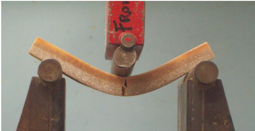
Figure 28: Flexural testing of CPF resin sample
