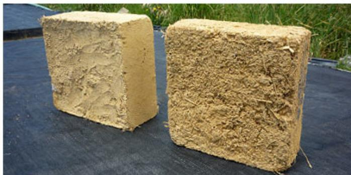
**Figure 1: Mud Brick; a simple composite material**
