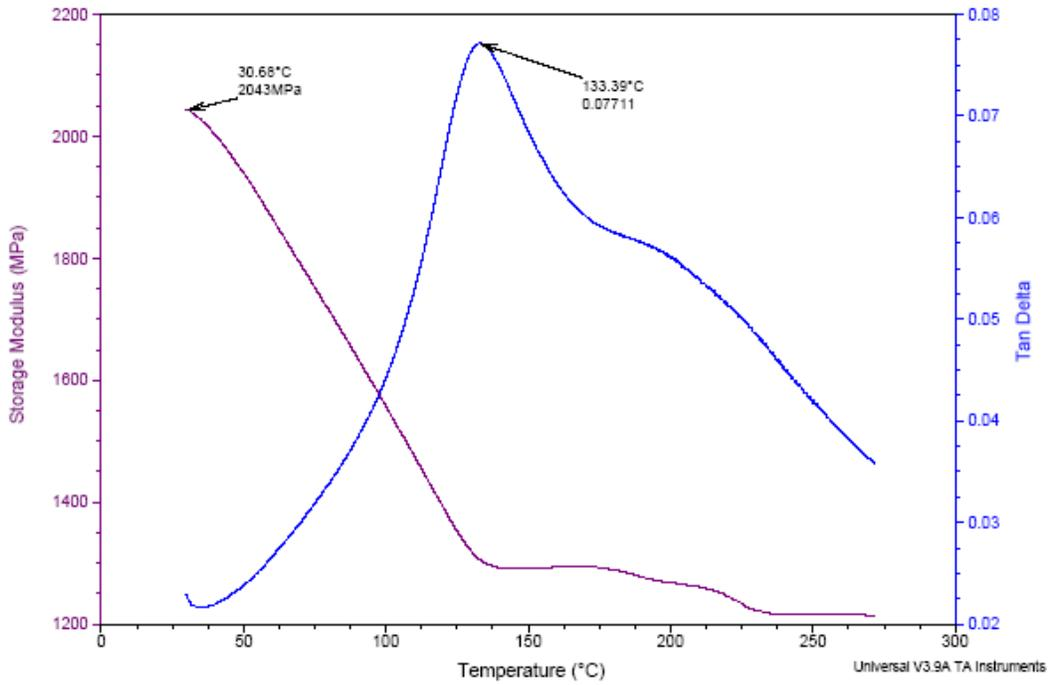
Figure 111: 100% PF resin - Wood fibre 10%
