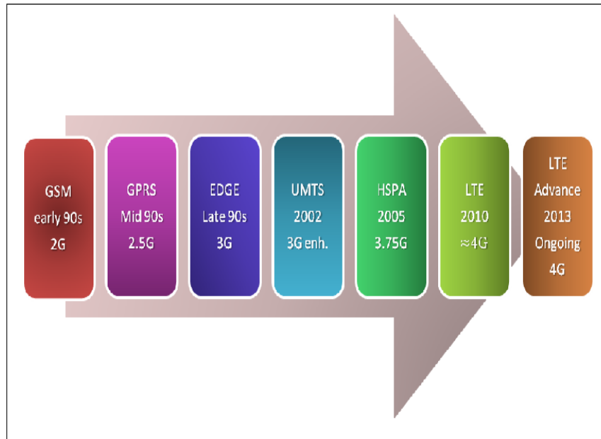
Figure 1: Digital Communication Standards System (this figure made using MS office power point)
