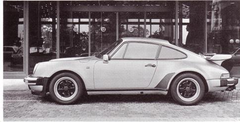
Figure 1.4: A Porsche 911. Note the aerofoil shape, and the large “Whale-Tail” rear spoiler (Hucho 1987).
