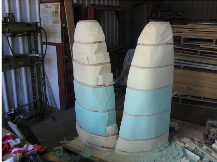
Figure 7.11: Comparison of rough-cut and sanded foam.
