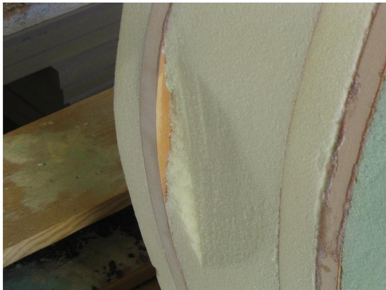
Figure 7.16: Care must be taken to avoid removing good material with the handsaw.
