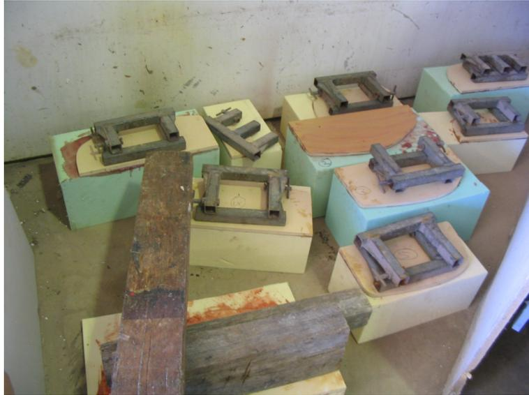
Figure 7.7: Each section was mated to a foam block and the resin allowed to cure before continuing.
