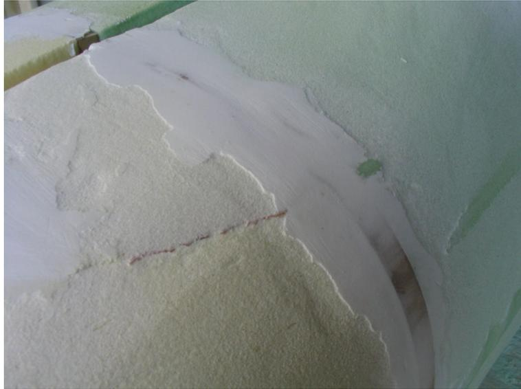
Figure 7.14: Eroded foam adjacent to the bog around the section 150mm forward of the front hoop.
