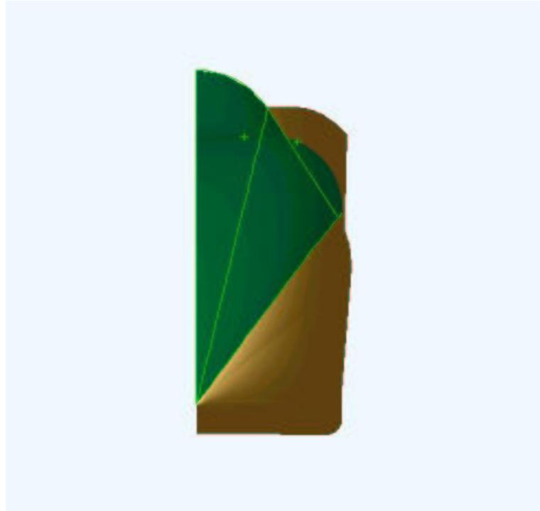
Figure 4.18: Front view of the face edges, showing them not bending tangentially to the bodywork surface along their length.
