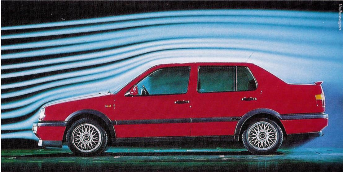
Figure 1.5: Smoke visualisation of streamlines along the centreline of a car in a full-scale wind tunnel (Edgar 2000).
