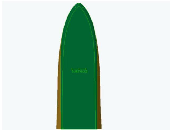
Figure 4.35: The floor of the nose, showing that its edges are not parallel aft of the bulkhead. Also visible is the change in radius of the fillet along the length of the filleted edge
