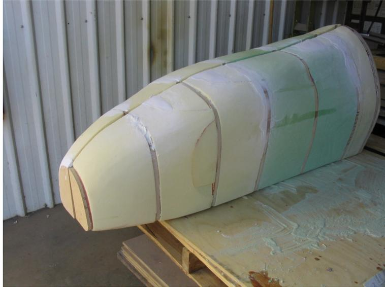
Figure 7.12: The partially bogged nose plugs side by side.
