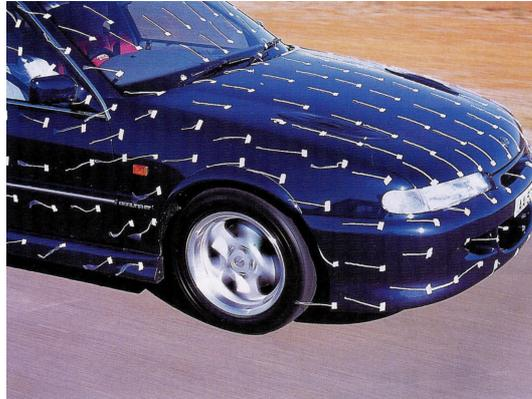
Figure 9.1: Wool-tuft testing a VR Commodore (Edgar 2000).
