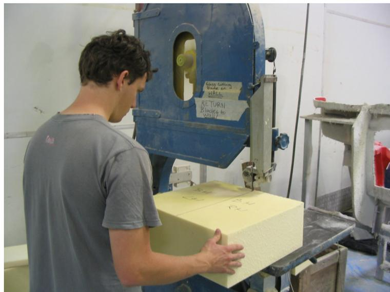
Figure 7.5: Brad Moody cutting the foam blocks on a bandsaw.
