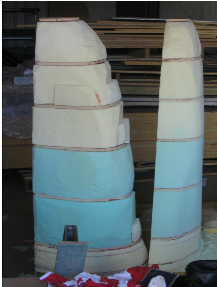
Figure 7.8: The blocks added to fill the gaps left by foam blocks that were too small.
