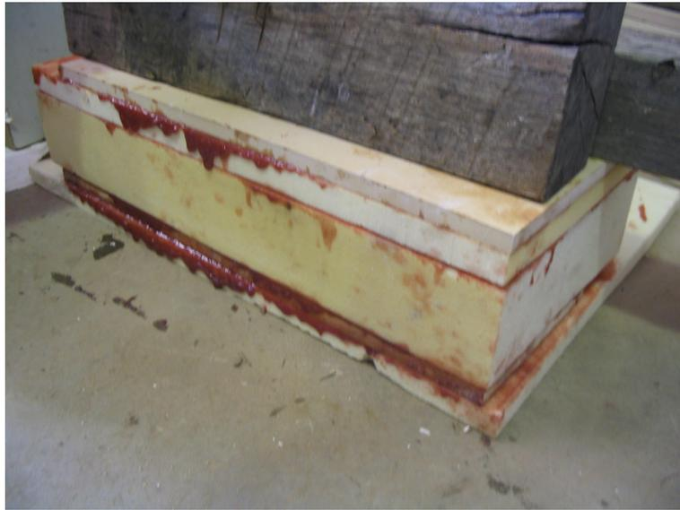
Figure 7.6: The near-failure. Four layers of wet resin allow floating of the parts before it cures.
