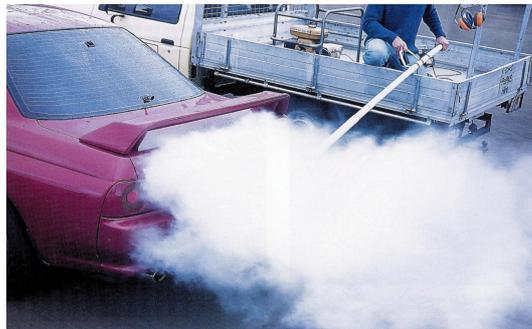
Figure 9.2: Smoke testing the wake behind an R32 Skyline (Edgar 2000).
