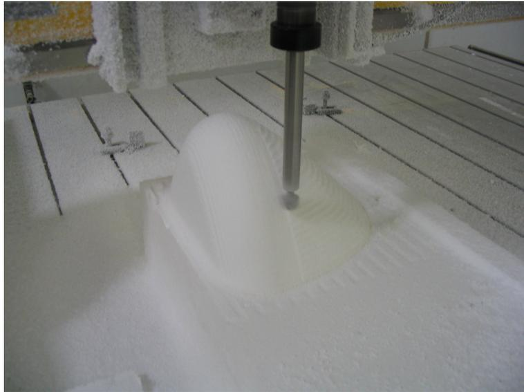
Figure 7.9: 130mm of nose cone being cut on the CNC machine.
