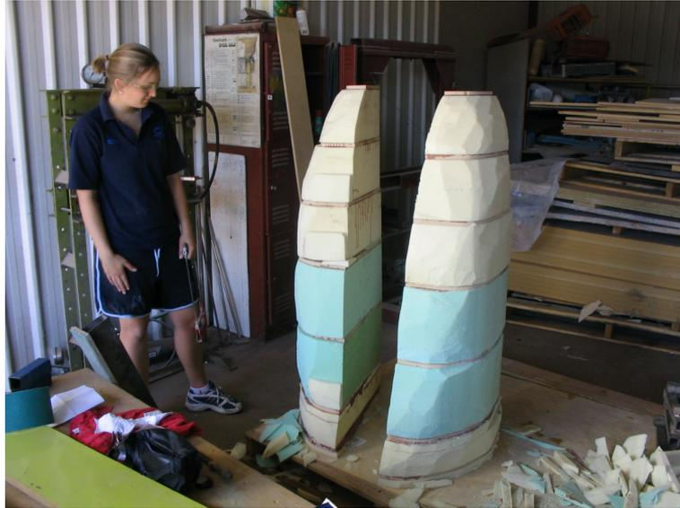
Figure 7.10: Vivienne French uses a handsaw to cut away unwanted material before sanding begins.
