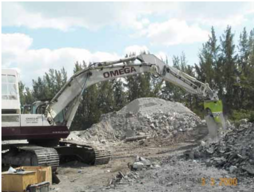
Figure 2.3: Hydraulic Crusher with Long Boom Arm (Source: Hydraulic Circuit Technology, 2000)
