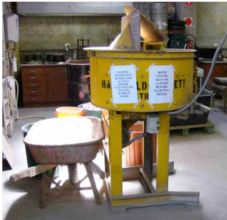
Figure 3.5: Horizontal Pan Mixer
