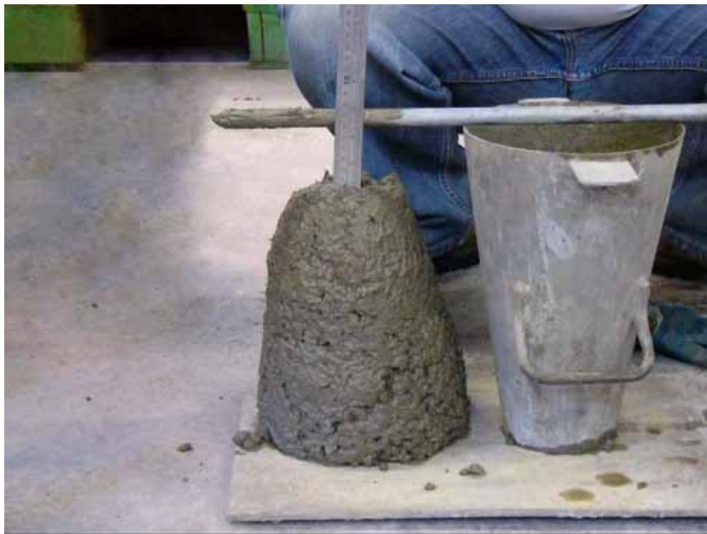
Figure 4.2: Typical Slump Test
