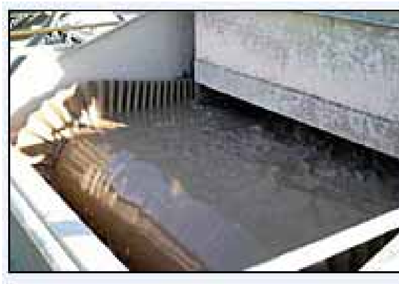
Figure 2.10: Wet Separation Process (Aquamator) (Source: Boral, 2002)
