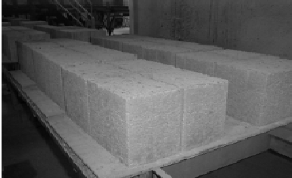
Figure 1.6: Recycled Aggregate used as Building Blocks (Source: Mehus and Lillestol (n.d))
