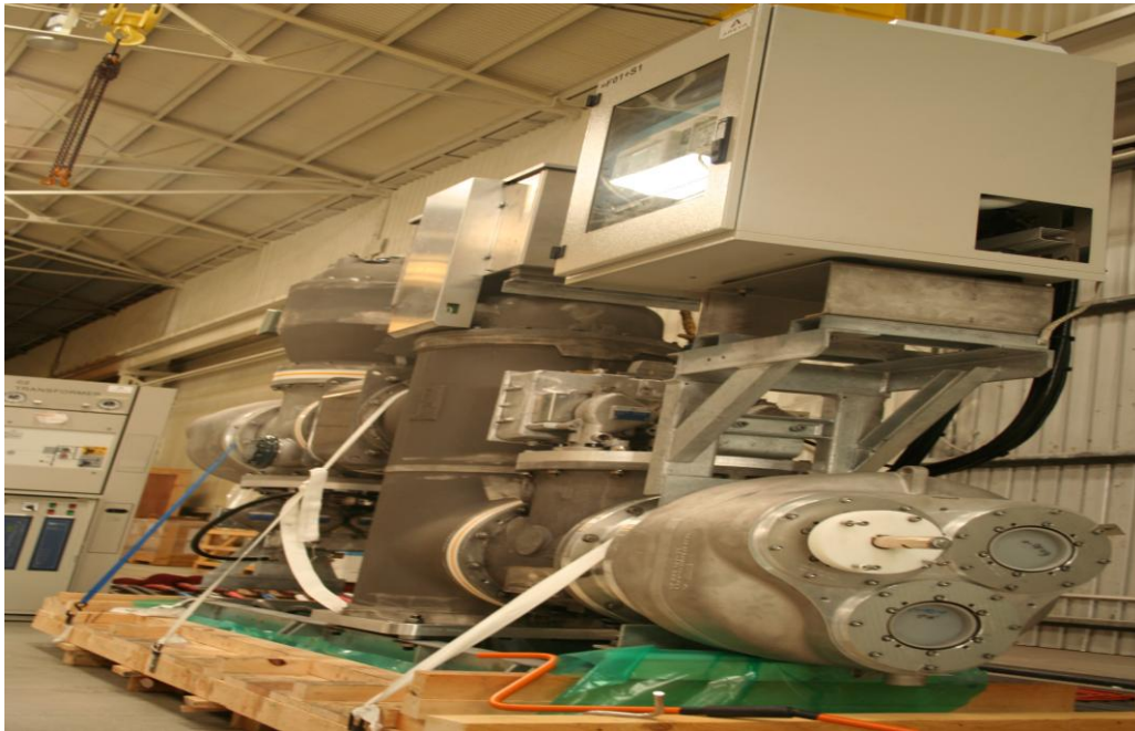
Figure 21: A relocatable GIS switchgear (Ergon Energy, 2011)
