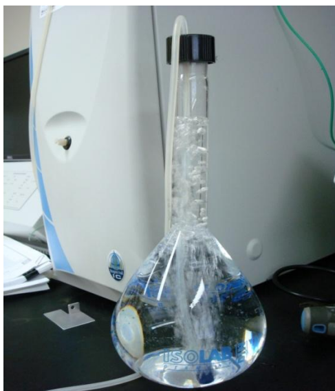
Figure 4.7: Helium sparging to remove dissolved oxygen
