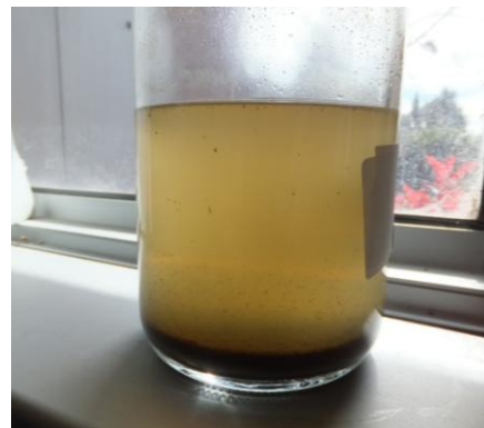
Figure 6.5: Saveall water: Final 10 days showing floating layer has been digested
