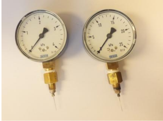
Figure 4.9: Pressure gauges fitted with hypodermic needles
