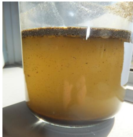
Figure 6.4: Saveall water: First 10 days showing floating layer on top
