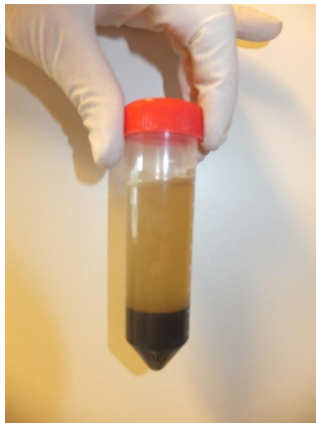
Figure 4.6: Anaerobic sludge after centrifuging showing pellet of inoculum
