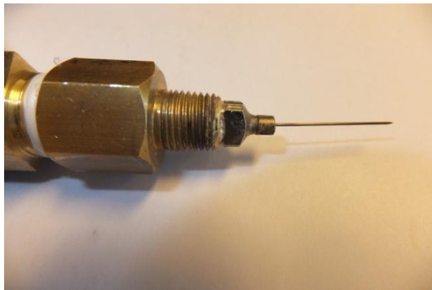
Figure 4.10: Close up of hypodermic needle connection
