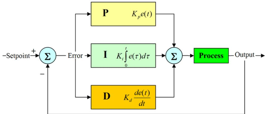
Figure 2.10: Basic PID control loop structure (SilverStar 2006)
