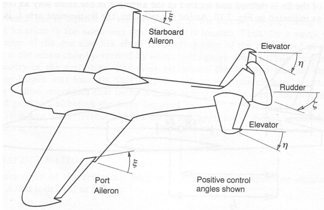
Figure 2.2: Control surfaces of a four axis aircraft (Cook 1997)
