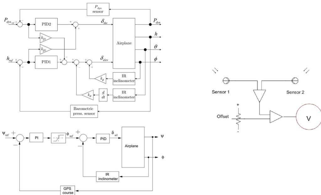
Figure 2.11: Comparison of control loop topologies left (Iscold et al. 2010), and right (Taylor et al. 2003)
