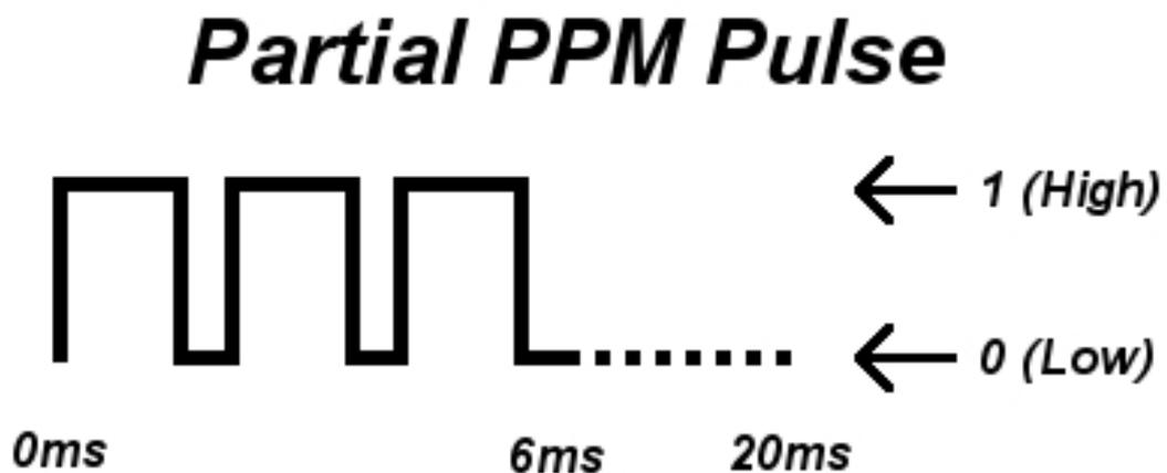
Figure 2.9: Using Pulse Position Modulation (PPM) to multiplex the servo control signals (Endurance RC 2010)
