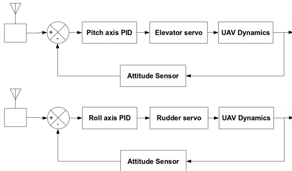
Figure 5.5: Control system block diagram (fly-by-wire mode)
