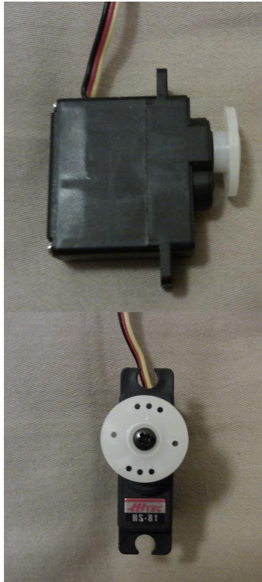
Figure 4.5: HiTec HS-81 servo motor
