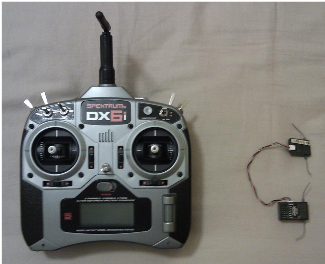
Figure 4.3: Spektrum DX6i remote control transmitter and receiver set
