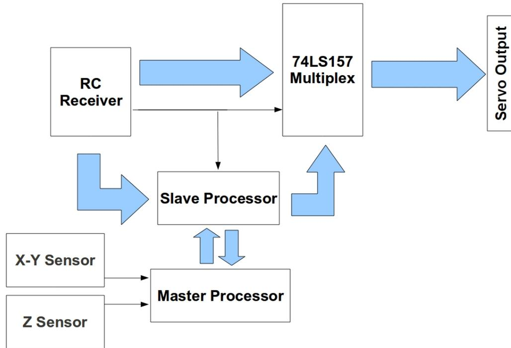
Figure 6.2: Introduction of a secondary processor to the control system
