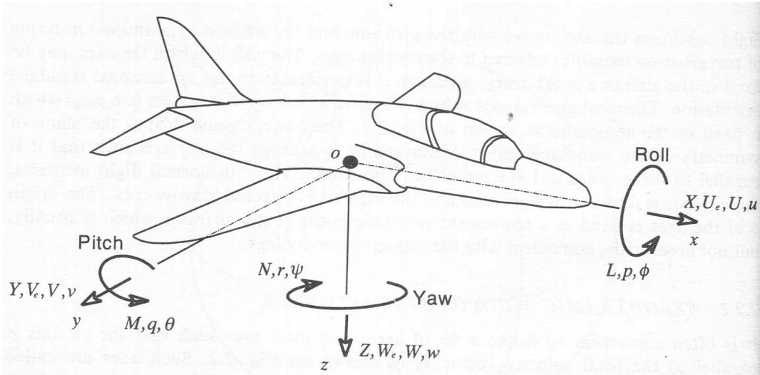
Figure 2.1: Definition of flight axes and variables (Cook 1997)
