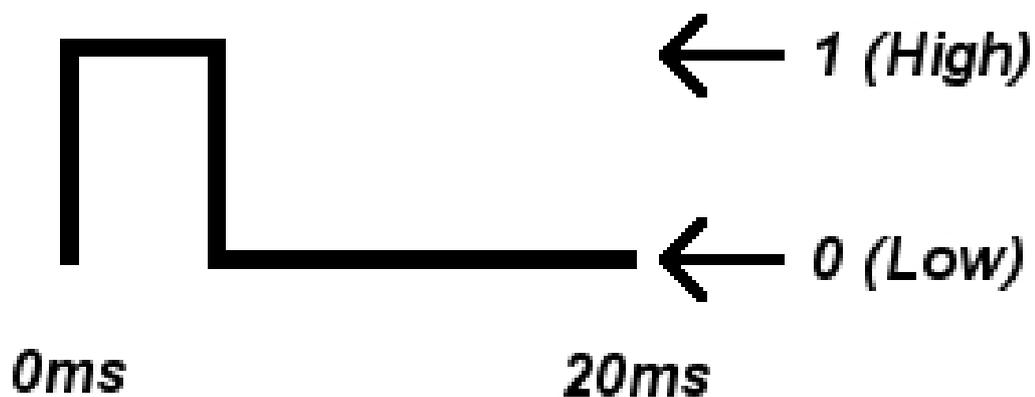
Figure 2.8: Servo motor control signal pulse (Endurance RC 2010)
