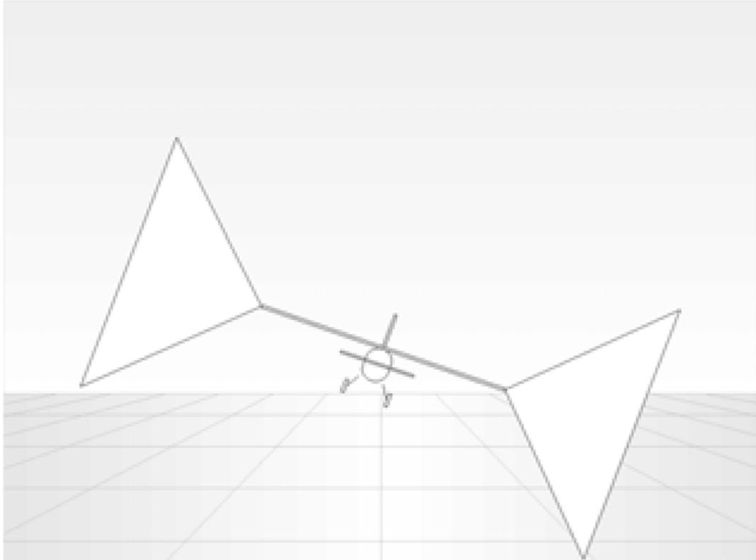
Figure 2.6: Thermopile sensor configuration for detecting the roll angle of an aircraft (Taylor et al. 2003)
