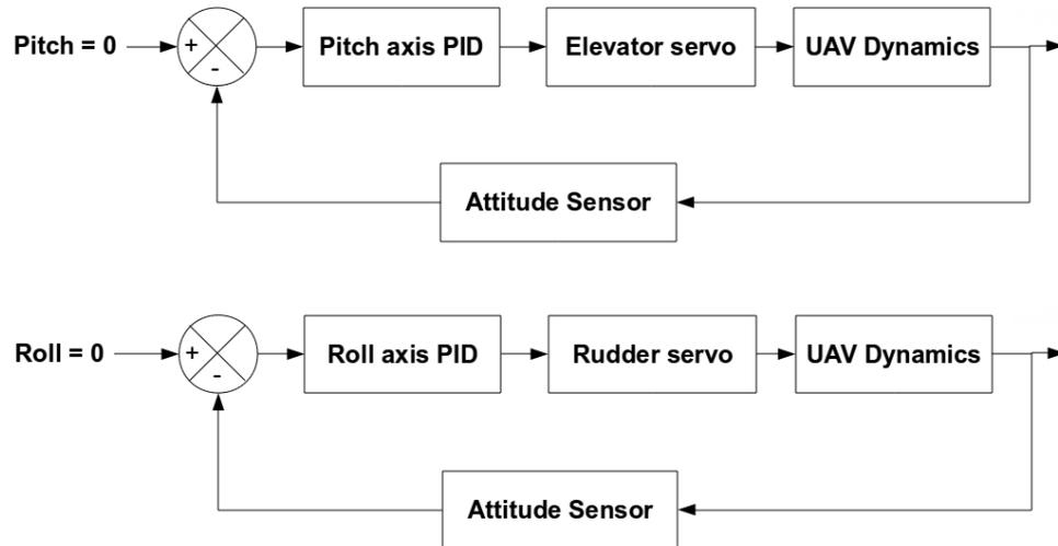
Figure 5.4: Control system block diagram (stabilisation mode)
