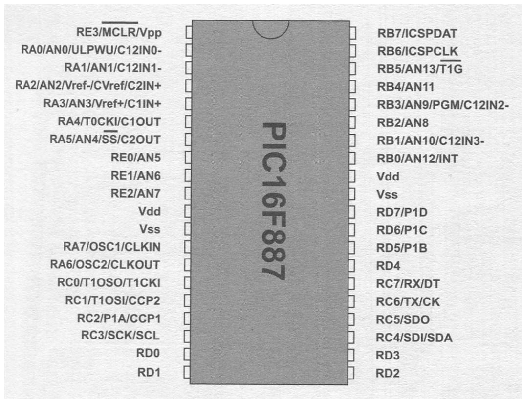
Figure 4.8: PIC16F887 pin out diagram (Verle 2008)
