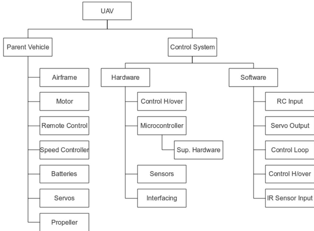
Figure 4.1: UAV system topology
