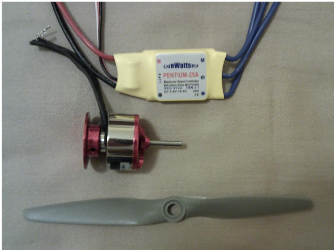
Figure 6.3: New brushless motor, speed controller and propeller
