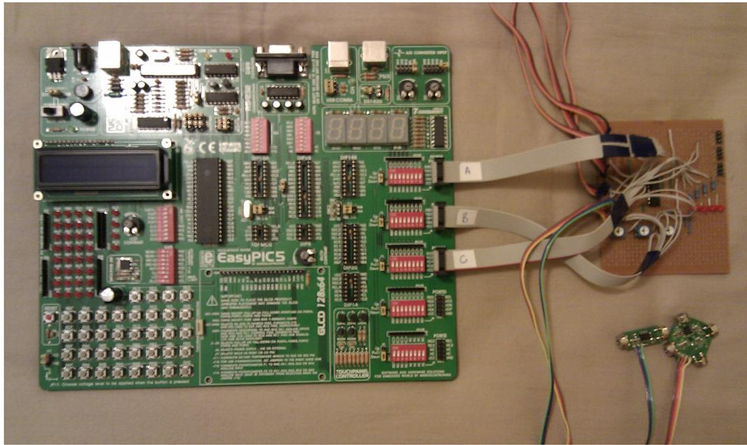
Figure 5.3: EasyPIC5 development board and UAV hardware prototype
