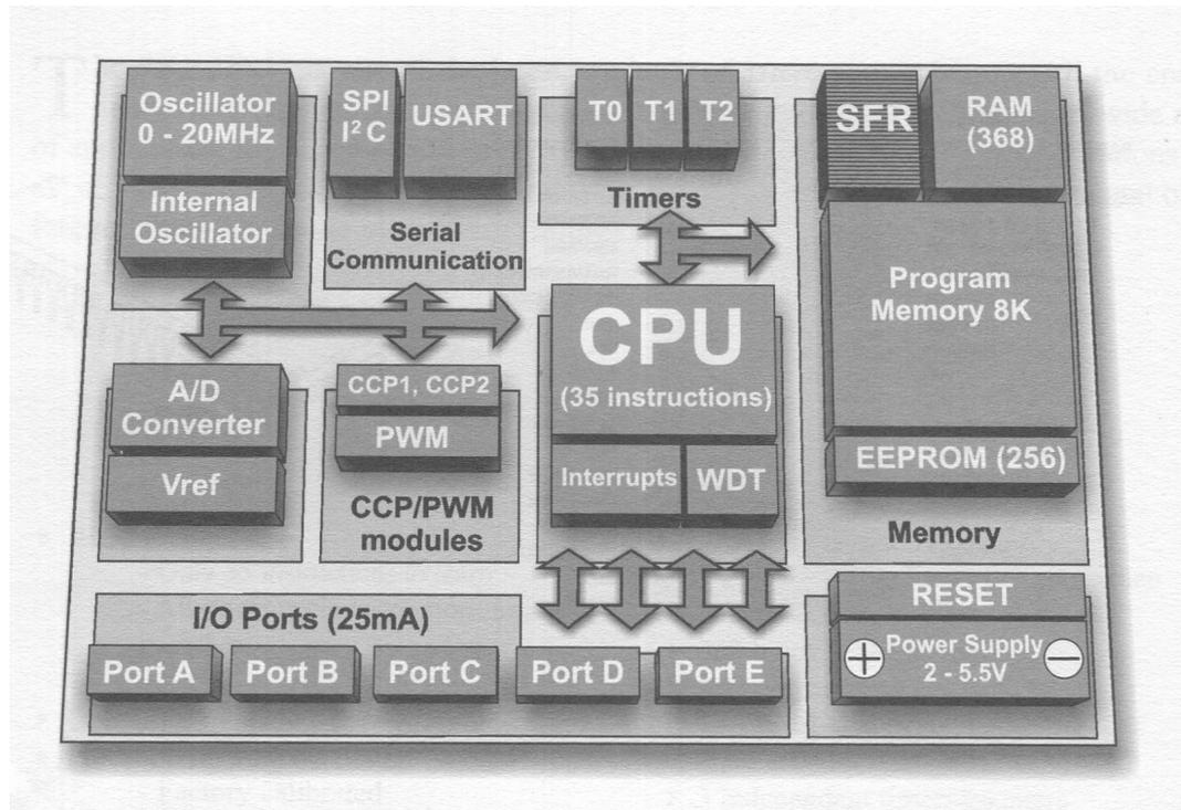
Figure 4.7: PIC16F887 internal block diagram (Verle 2008)
