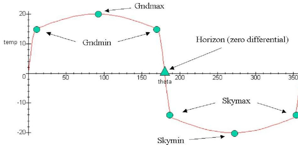
Figure 2.7: Revised model of temperature relative to roll angle for infrared thermopile sensors (Egan & Taylor 2007)
