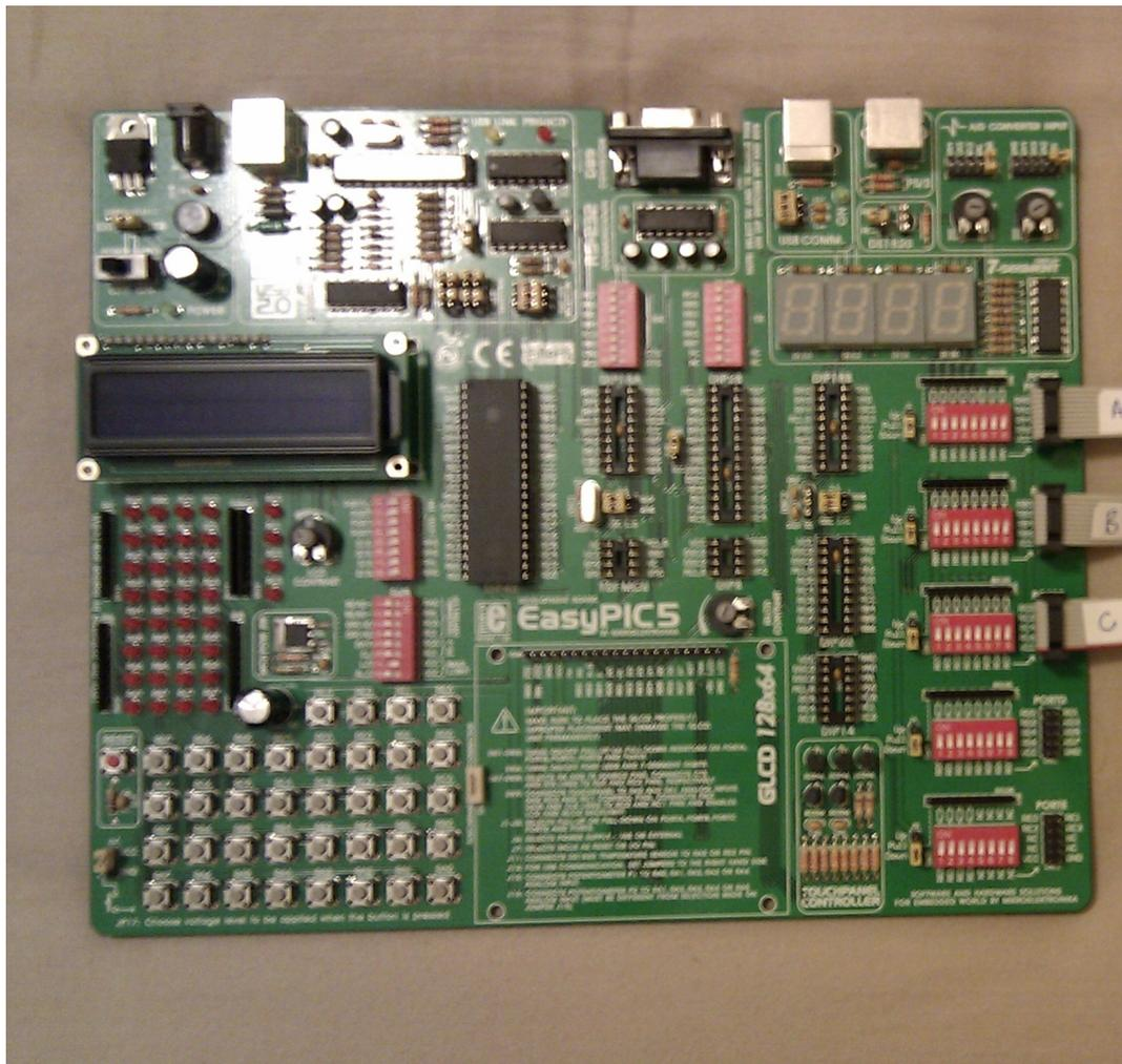
Figure 4.6: MikroElektronika EasyPIC5 Development Board
