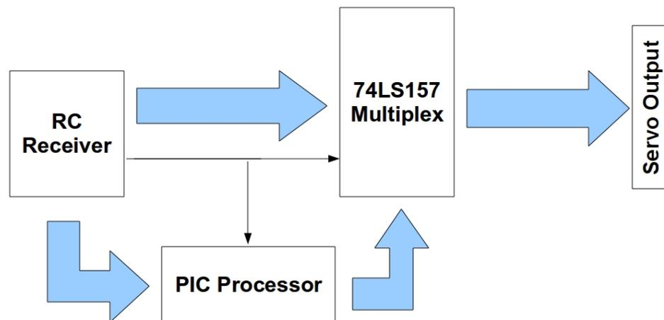
Figure 6.1: Revised control handover process using the 74LS157 multiplexer
