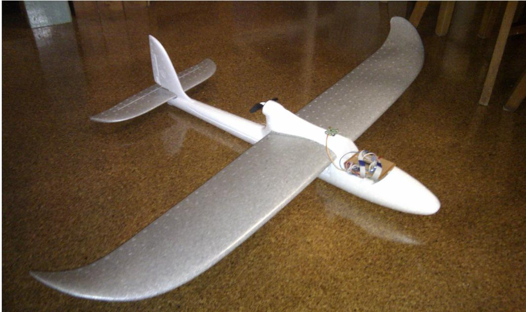
Figure 4.2: Multiplex EasyStar remote control foam glider (shown with control system fitted)
