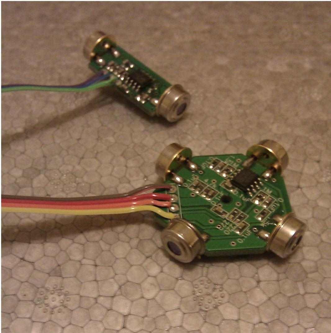
Figure 5.2: Infra-red thermopile sensor boards
