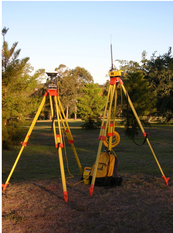
Figure 2.6 GPS base station setup.
