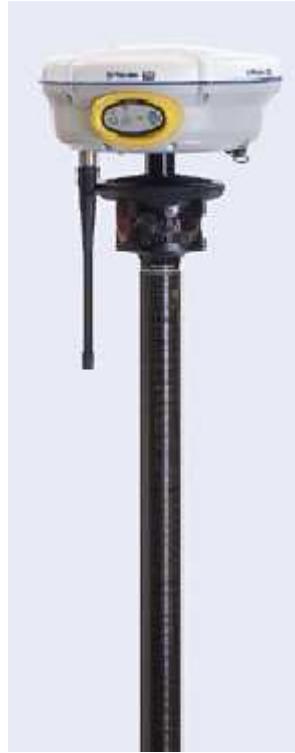
Figure 2.7 GPS and S6 prism attached to same pole
