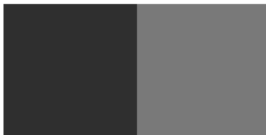
Figure 5.9: The ideal blur test image. It is simply a two square checkerboard 400 by 200 pixels. Note the grey values used to colour the squares are not black and white.
