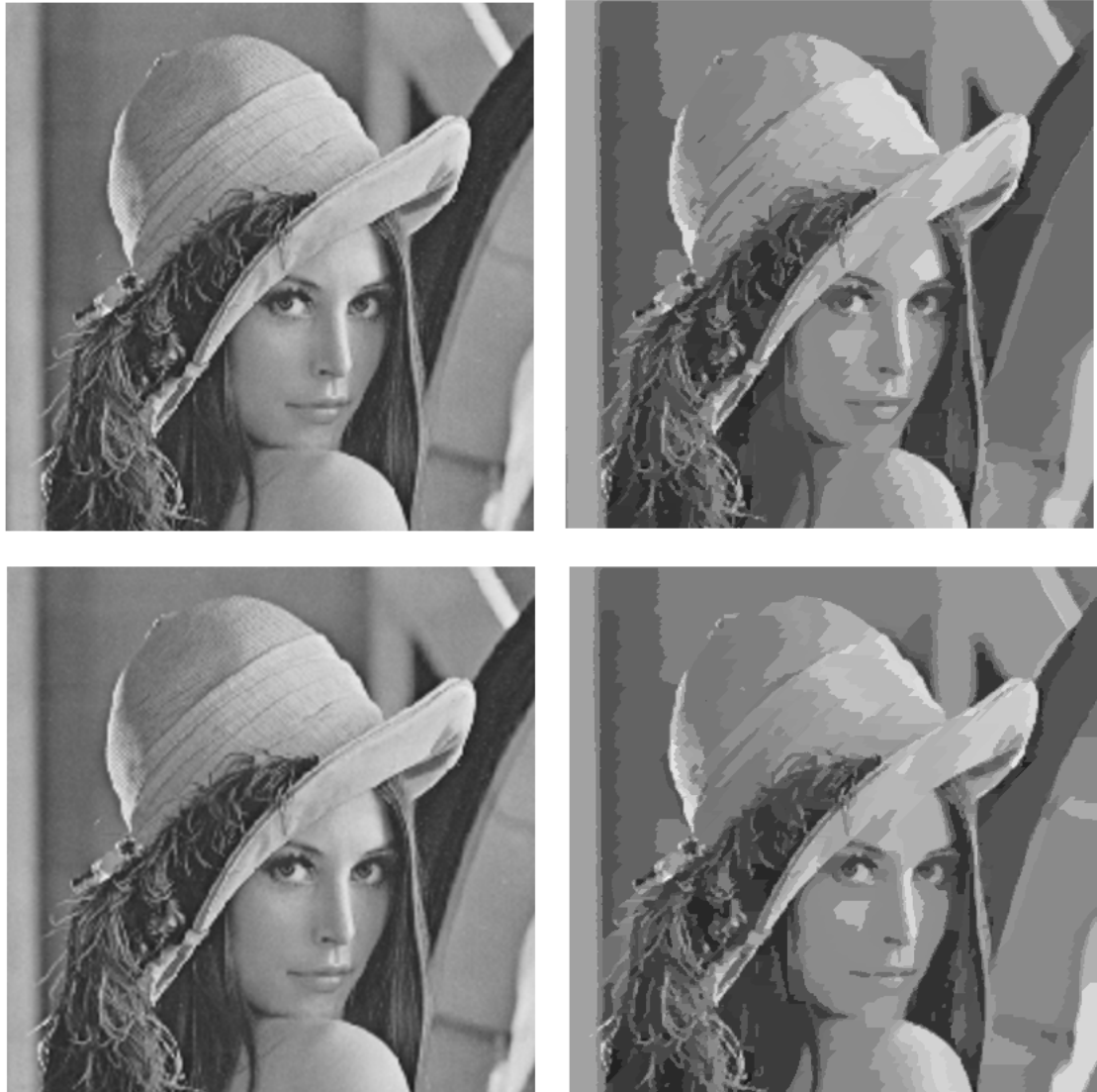
Figure 5.3: Illustration of the differences between two segmented images. The top set is 2% smaller than the bottom set. Notice the region discrepancies, especially in the foreground.
