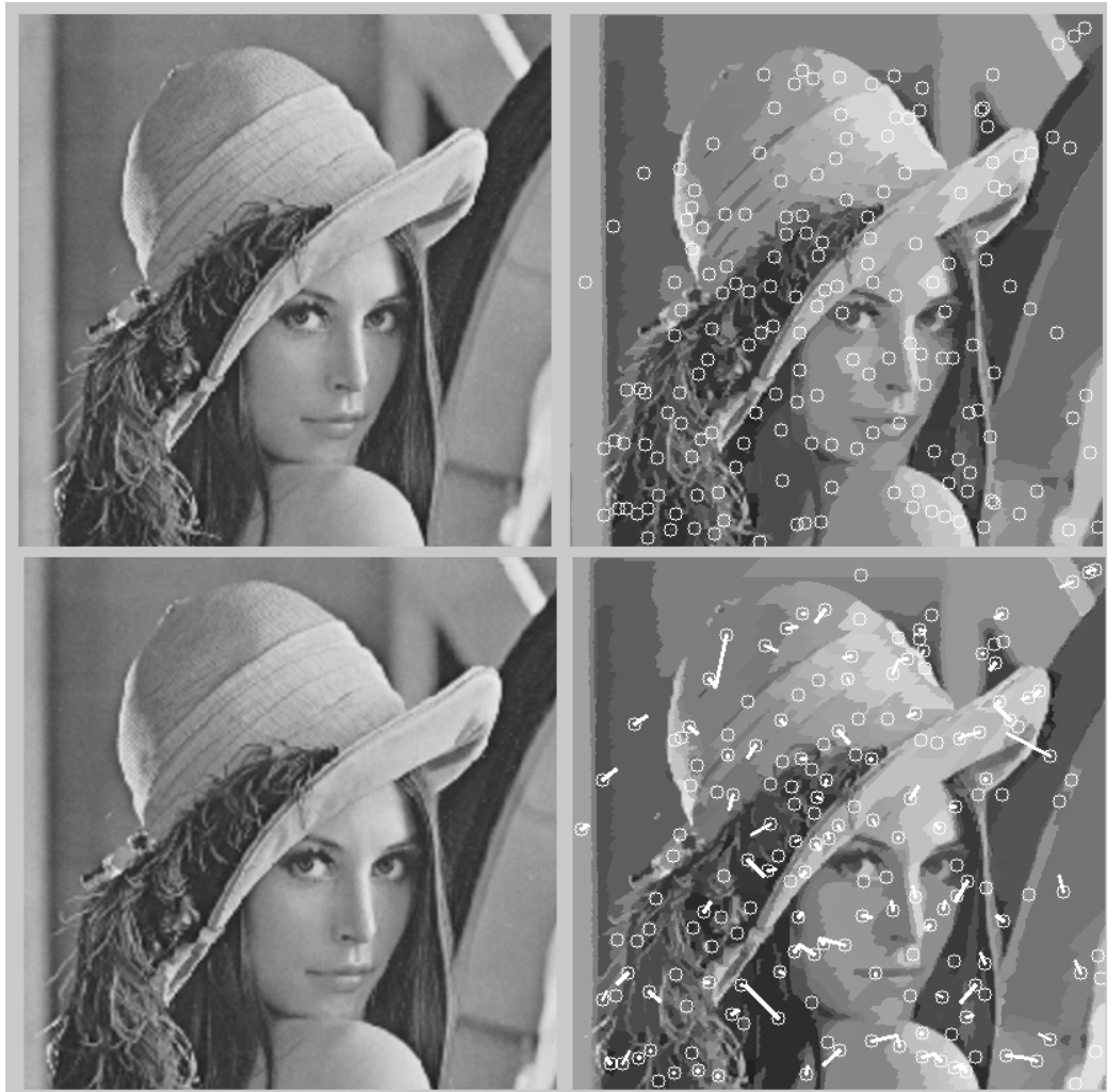
Figure 5.8: The results of tracking the segmented images in figure 5.3. The line from each centroid indicates the calculated position of that region in the previous frame.
