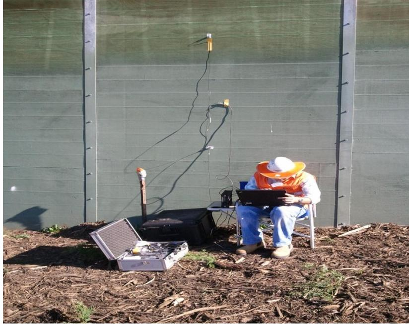
Figure 22 Equipment set up on Plywood Noise barrier
