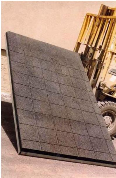
Figure 7 Recycled rubber barrier (<http://www.fhwa.dot.gov/environment/keepdown.htm>)
