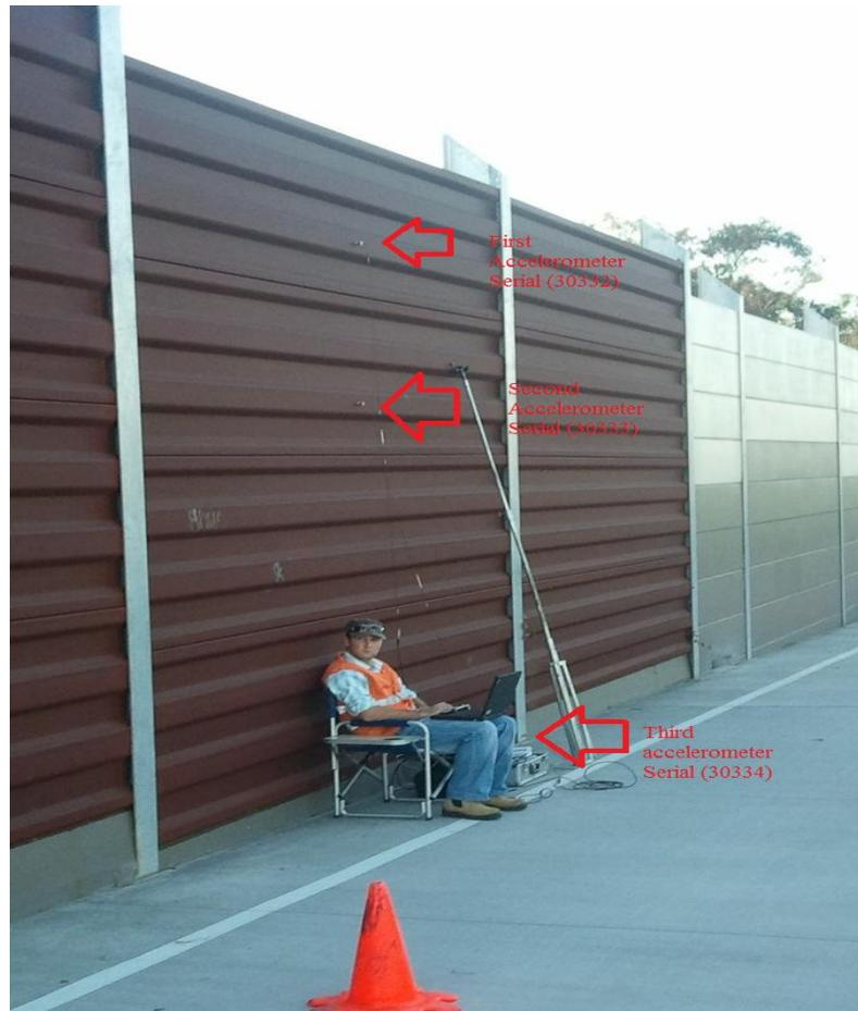
Figure 21 Accelerometer location on panels.
