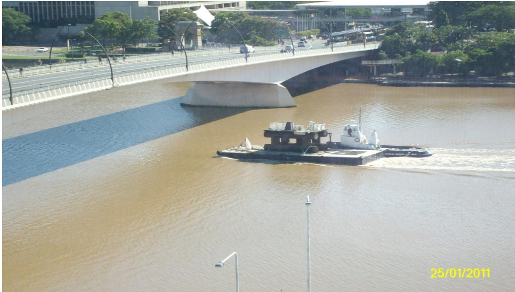
Figure 4-4 small flat top barge used for transporting salvaged materials to Fisherman's island
