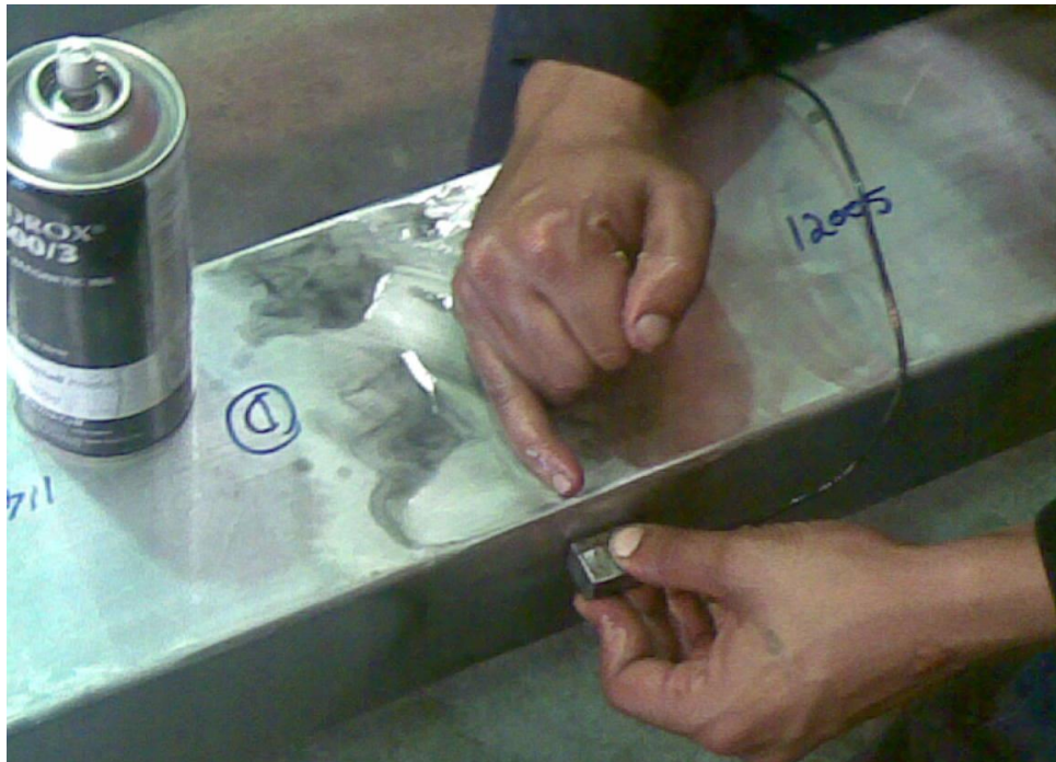
Figure 4-10 Ultrasonic testing of welds on Gangways
