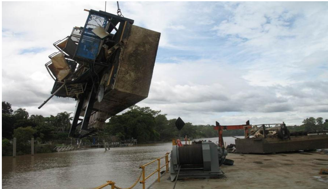
Figure 4-5 Retrieval of sunken pontoon from Brisbane river during the 2011 flood, being loaded onto the 'Maeve Anne'
