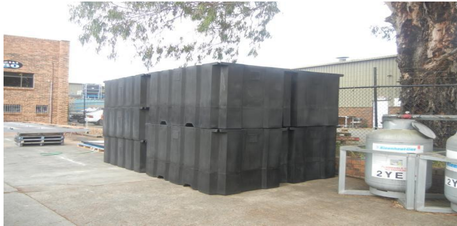
Figure 4-15 floatation modules used to construct pontoon for QUT terminal
