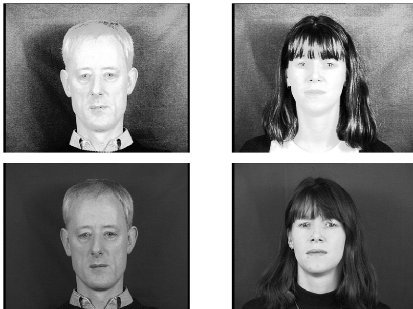
Figure 8.8: Histogram equalisation (top) in comparison to the original image (bottom)
