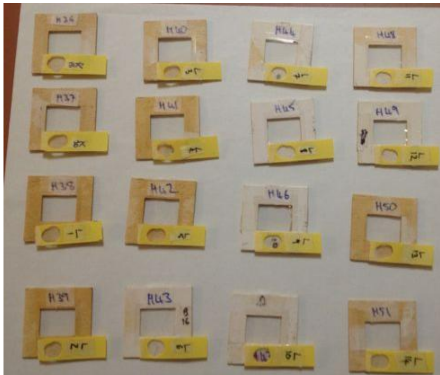
Figure 12 Paired large and miniaturised dosimeters prior to placement on plants or head forms
