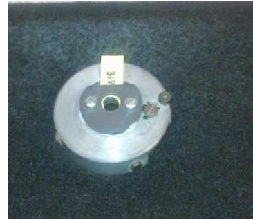
Figure 8 Miniaturised dosimeter in holder attached to mount
