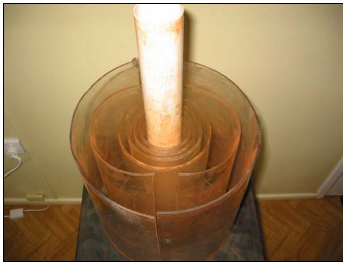
Figure 3-3 Sleeves surrounding access tube showing the largest 2 sleeves cut along their length
