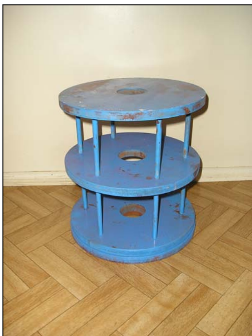
Figure 3-5 Tool used for compacting soil into the largest diameter sleeve
