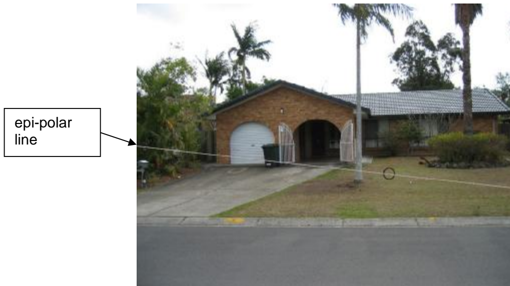
Figure 3.4 – Photograph showing epi-polar line crossing placed control marks
