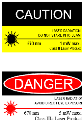
Figure 7.1: Typical warning label to be used with laser equipment. Source: “AR-600 data sheet” from www.acuityresearch.com
