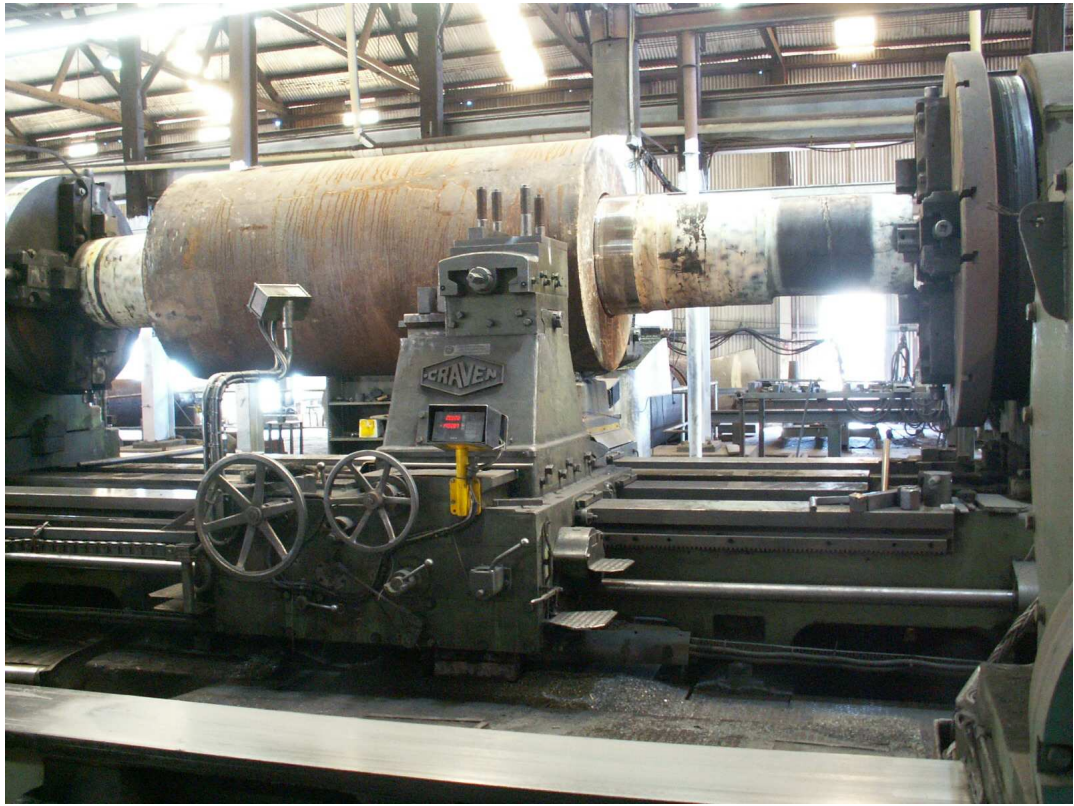
Figure 2.4: About to commence cutting the grooves in a shell
