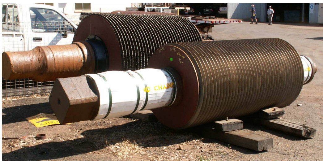
Figure 2.5: Two completed rollers. The rear roller has arcing, the front one does not.
