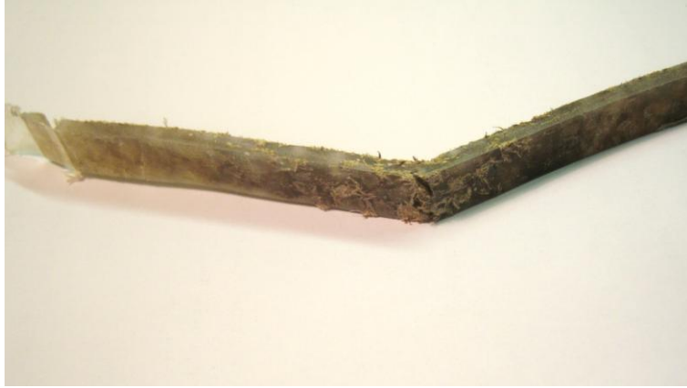
Figure 10: Flexural testing - breakage at fibre clump
