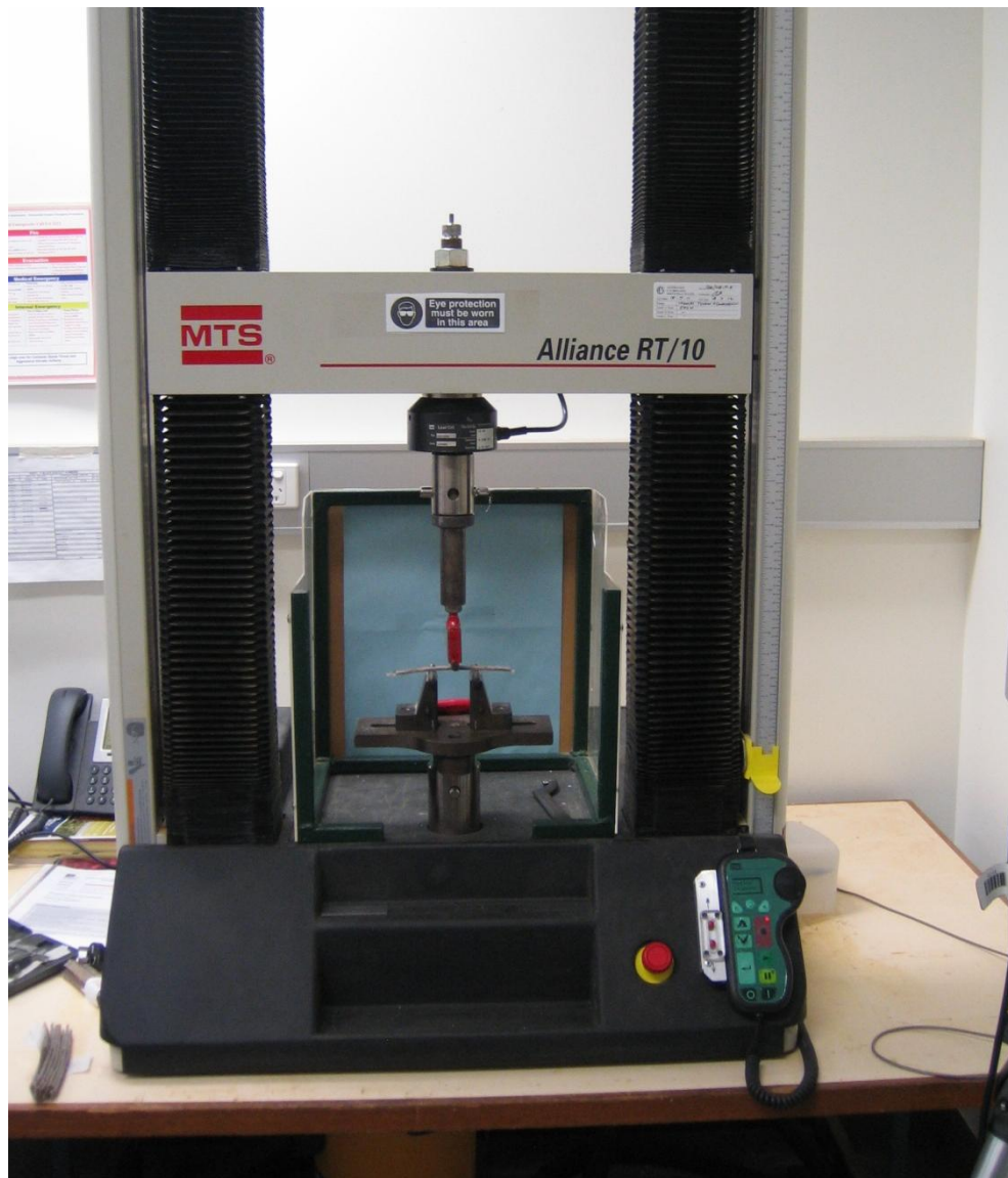
Figure 5: Three-point flexural testing set up
