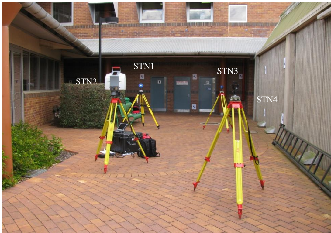
Figure 3.2-1: USQ TLS calibration showing station positions
