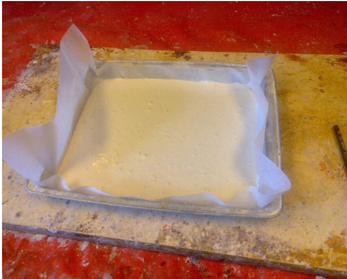
Figure 3.1: The mould for casting flexural test sample
