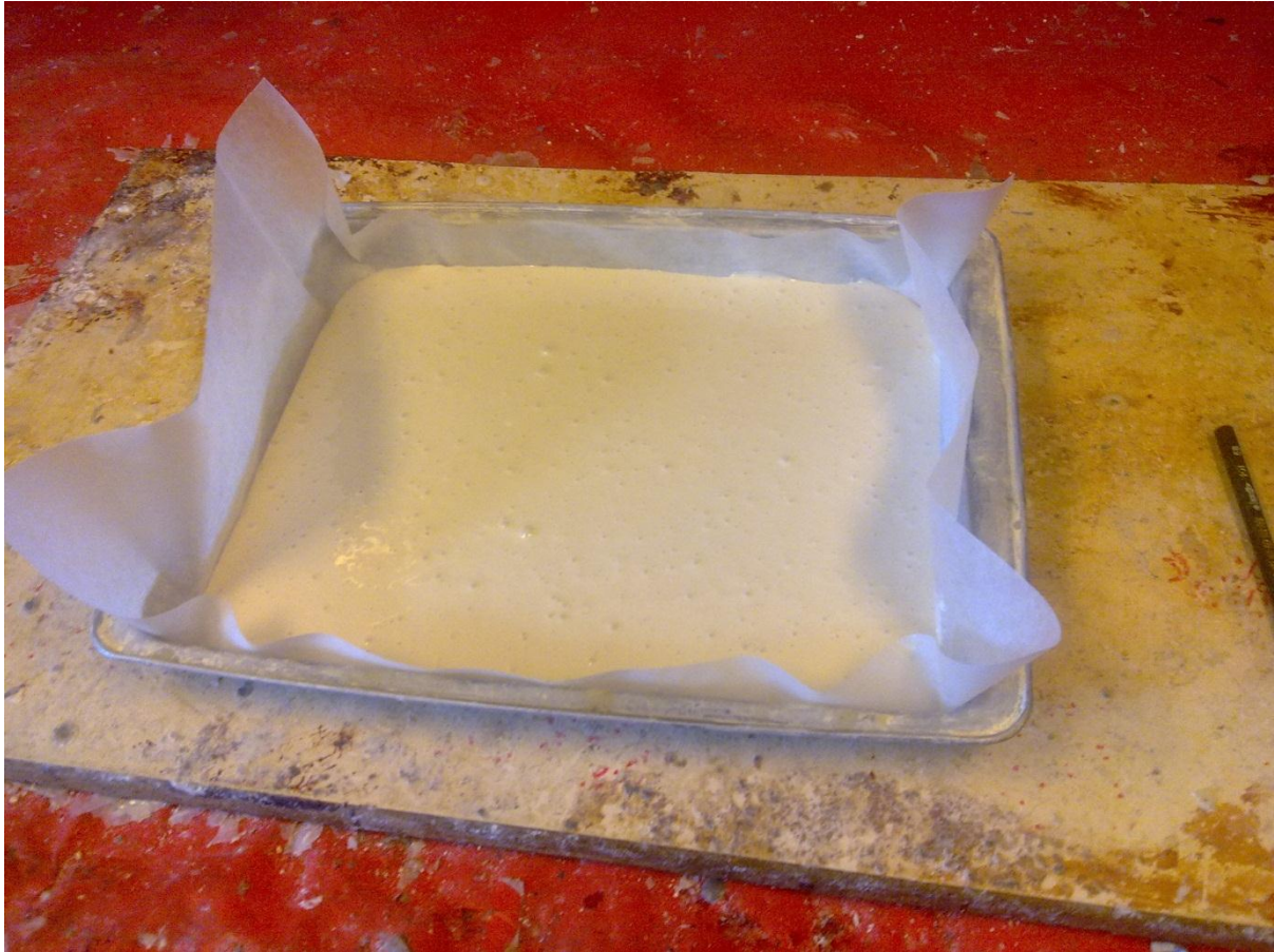
Figure 3.7: The mould used to cast flexural test specimens.
