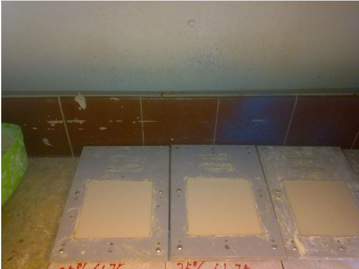
Figure 3.2: The mould used for casting the samples for loss tangent test and thermal analysis
