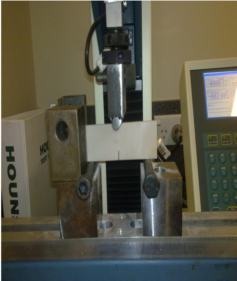
Figure 3.9: Specimen loaded onto Hounsfield testing machine
