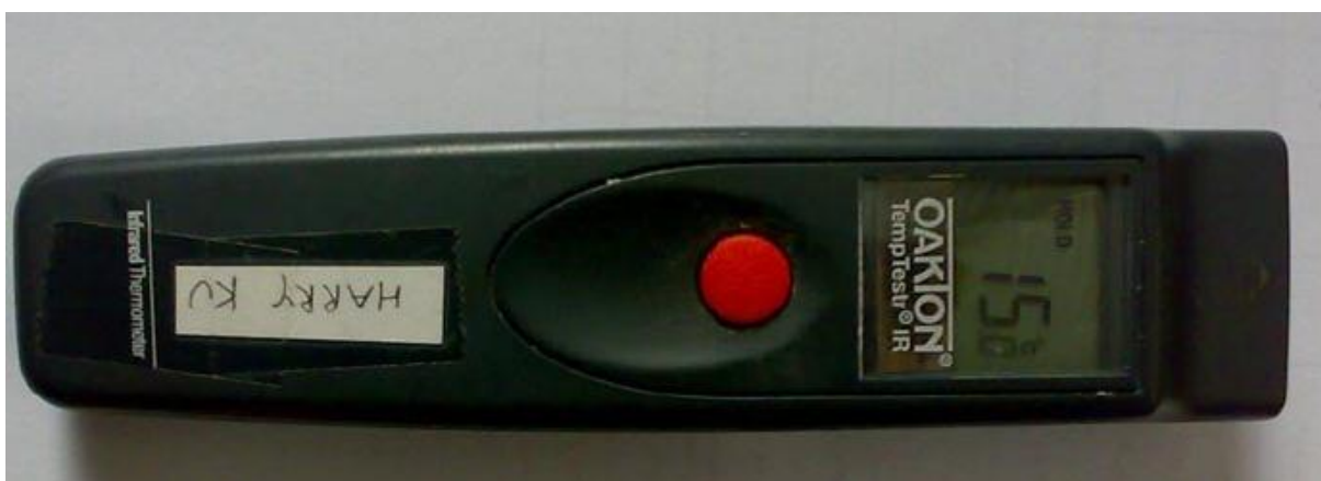
Figure 3.6: The infra-red handheld thermometer
