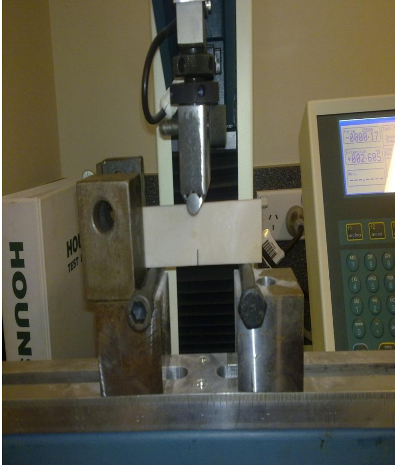
Figure2.6: Three-point loading system on a Hounsfield testing machine
