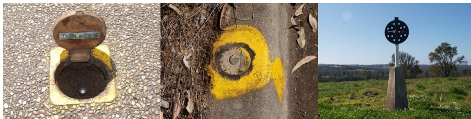
Figure 3.3-Class LC or higher permanent marks used in study
