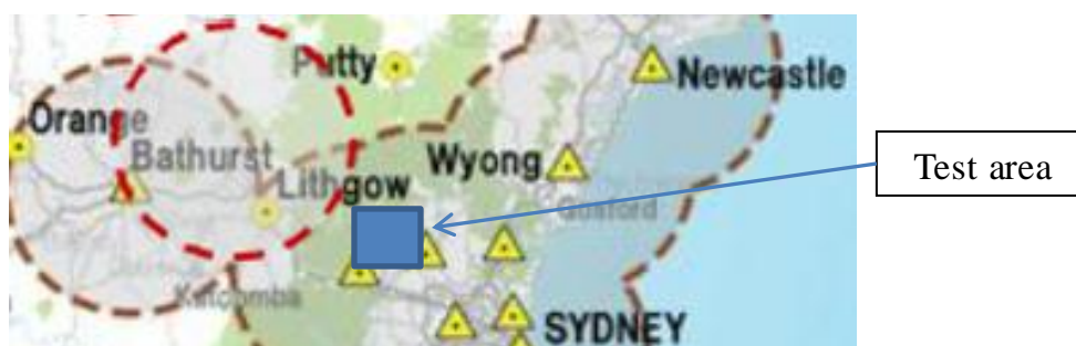
Figure 3.2-Circles indicate 50km operating range of CORSnet reference stations. The Putty and Lithgow reference stations have become operational since this publication (image source Department of Lands 2009)
