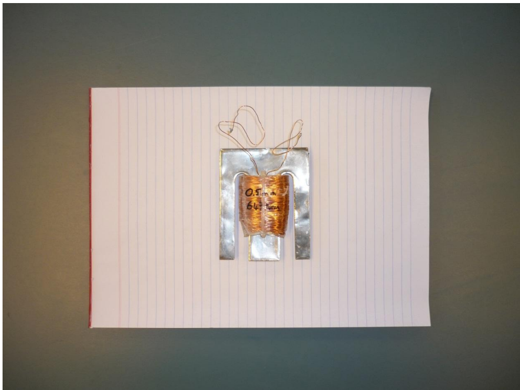
Figure 33. Produced Magnetostrictive Transducer by W.A. McHugh on an A4 Sheet of Paper.
