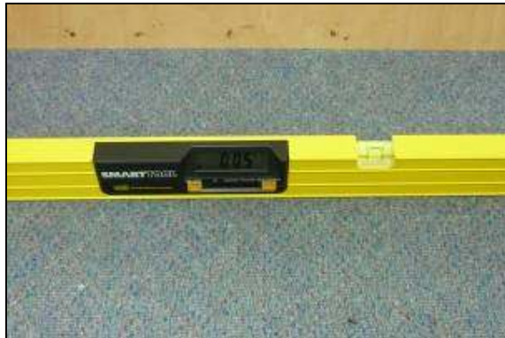
Figure 6.2: Digital level used in estimating road crossfall
