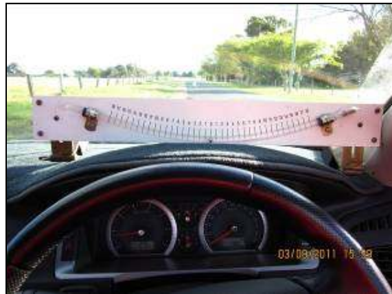
Figure 6.4: Ball bank indicator in survey vehicle
