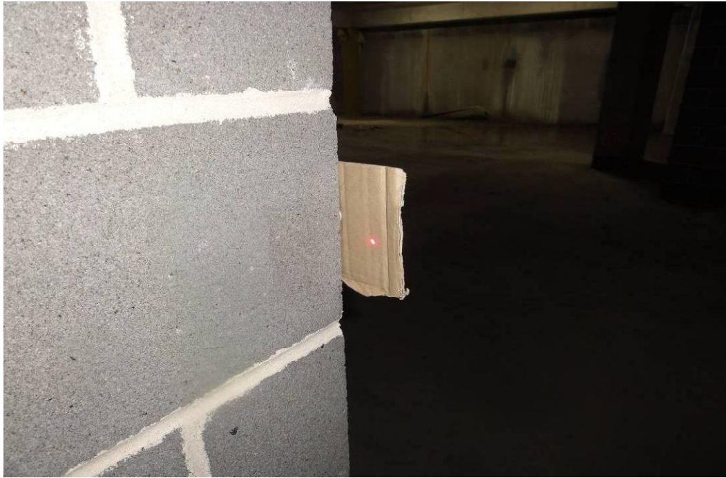
Figure 5.4: Temporary Cardboard Reflector and Blu-tak. (Note the Laser dot)
