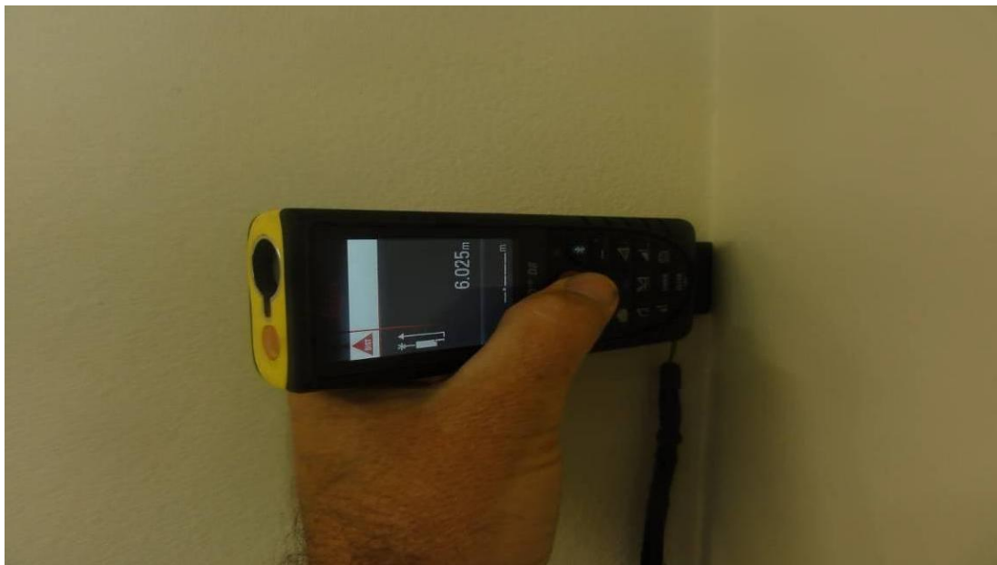
Figure 5.3: Leica Disto D8 showing third measure point at an internal corner
