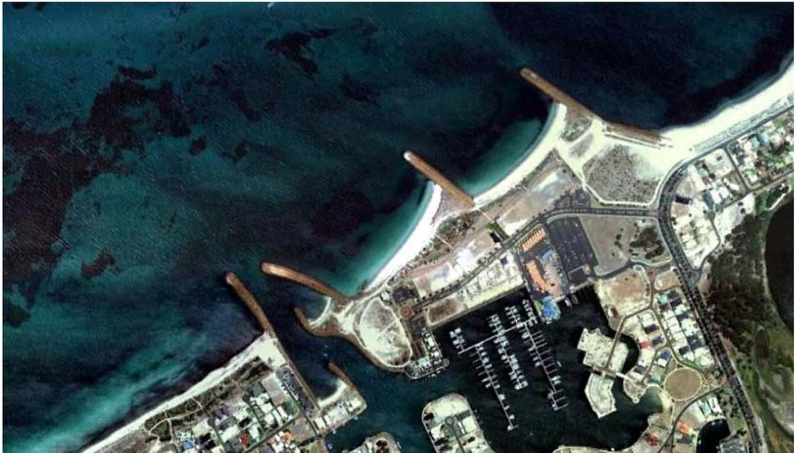
Figure 12 – Accretion & Erosion at Port Geographe due to Groynes – 2010 (Google Earth 2011)
