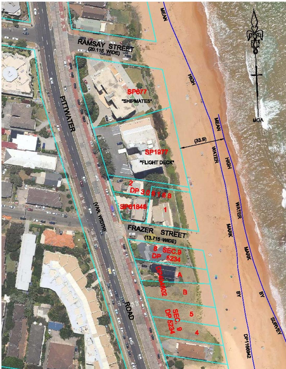
Figure 22 – Position of Mean High Water Mark as per survey & DP1166942 (background image – nearmap 2011)
