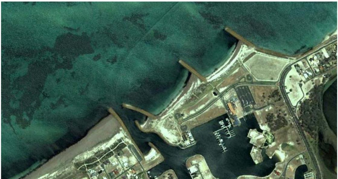
*Figure 10 – Accretion & Erosion at Port Geographe due to Groynes – 2003 (Google Earth 2011)*
