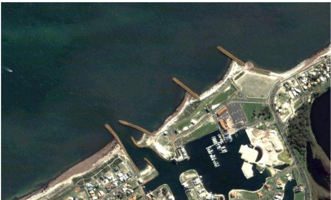
*Figure 11 – Accretion & Erosion at Port Geographe due to Groynes – 2005 (Google Earth 2011)*
