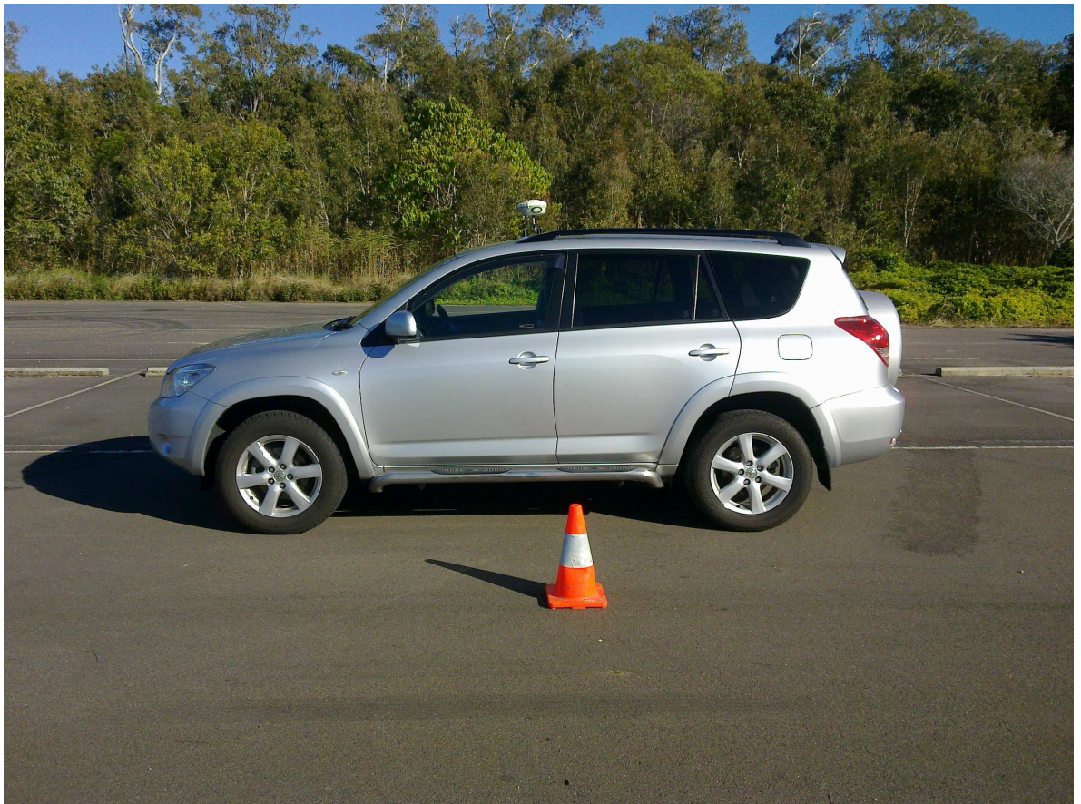
Figure 3.2 The set up of the latency test with the GNSS receiver mounted on the car roof
