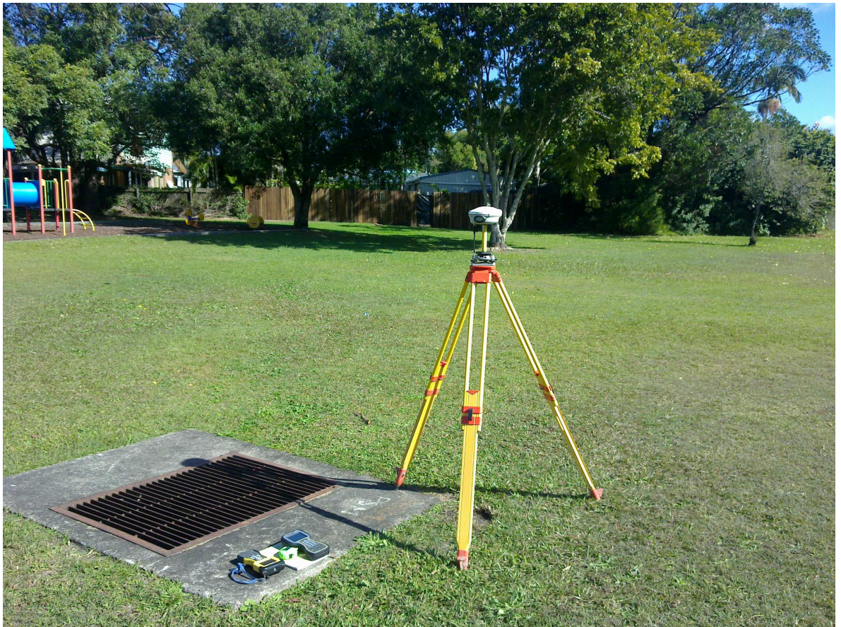
Figure 3.1 The set up of the static point measurement technique at PSM 103109
