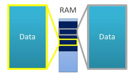
Figure 4.2 Representation of memory usage of two threads in a single process
