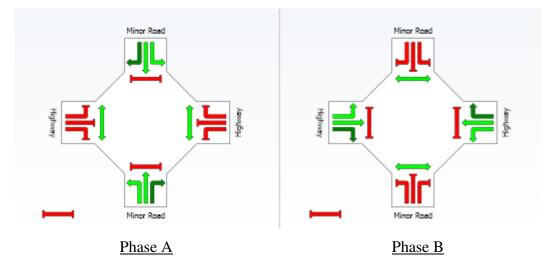
Figure 3.10: MATLAB Simulation Phasing Diagram
