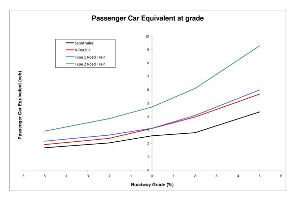
Figure 4.2: Impact of Grade on Passenger Car Equivalent Values
