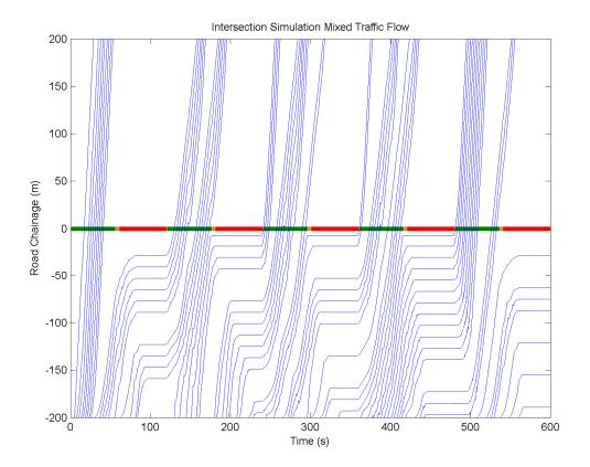
Figure 3.11: Simulation Output of Vehicle Position
