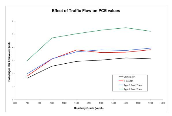
Figure 4.3: Impact of Traffic Volume on Passenger Car Equivalent Values
