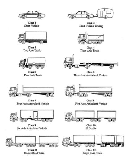
Figure 2.1: Austroads Representative Vehicles (Source: Austroads, 2009)
