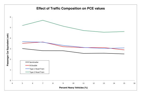
Figure 4.4: Impact of Traffic Composition on Passenger Car Equivalent Values
