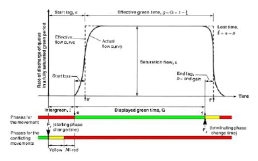
Figure 2.6: Traffic Signal Capacity (Source: Akçelik, 1998)
