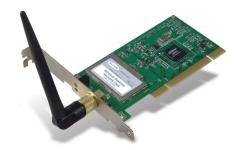
Figure 5.3: BELKIN High-Speed Wireless G Desktop Network Card.
