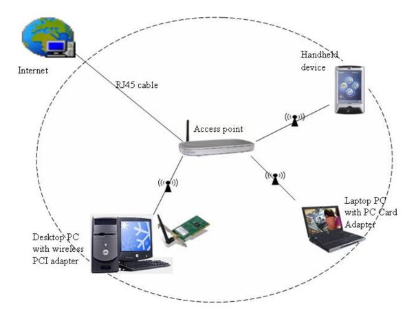
Figure 5.6: Topology design of desired Wireless LAN Testbed.
