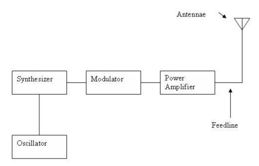
Figure B.3: Transmitter block diagram. Adapted from (Olexa 2005)
