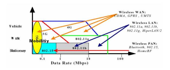
Figure 3.4: Overview of Wireless Networks (adapted from (Baghaei 2003)).
