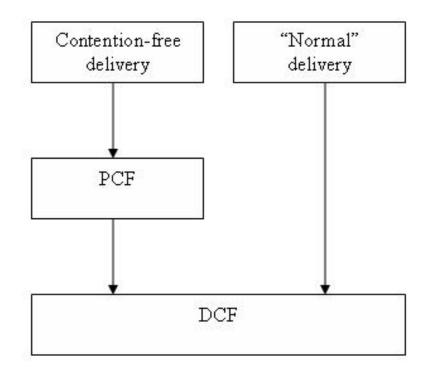
Figure 2.3: MAC coordination functions. (adapted from (Gast 2002)).
