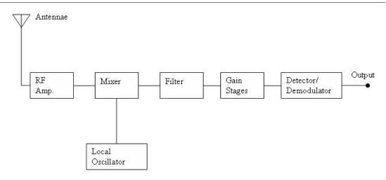
Figure B.4: Receiver block diagram. Adapted from (Olexa 2005)
