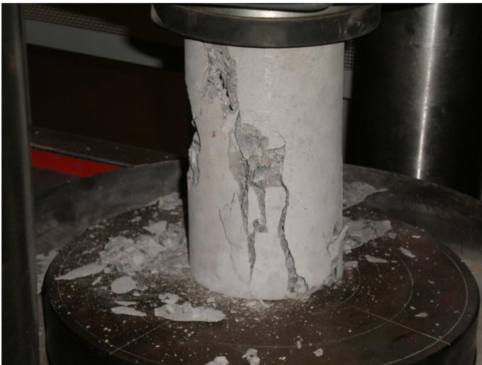
Photo 2 – Specimen 1 at failure
