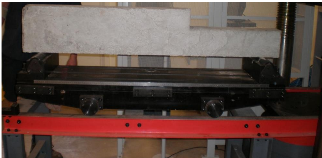
Figure 4.16 Specimen set-up on flexure grip
