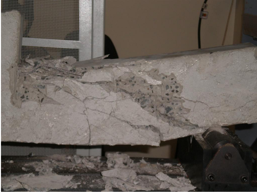
Photo 7 – Failure of optimum beam
