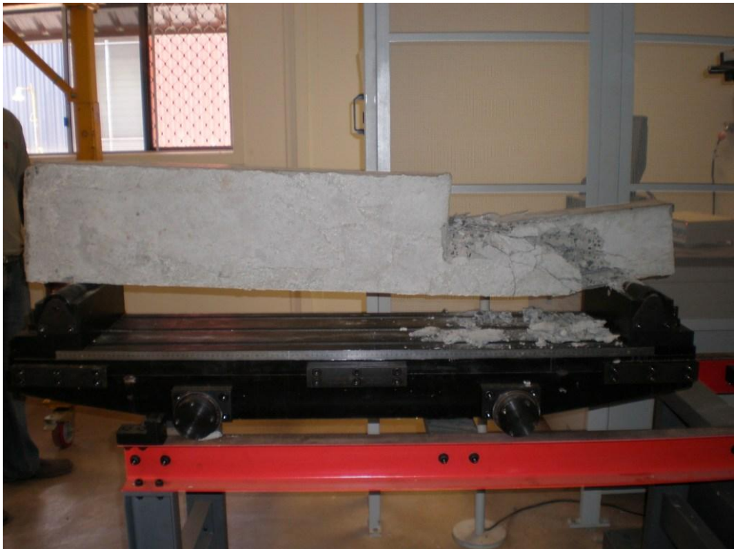
Photo 8 – Optimum beam at failure
