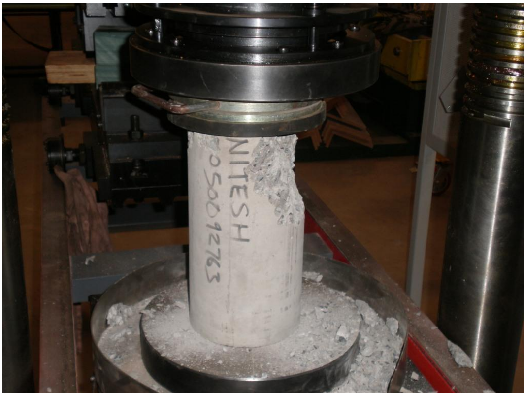
Photo 4 – Specimen 3 at failure
