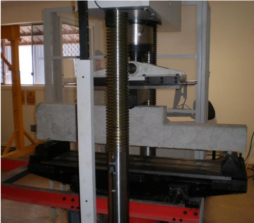
Figure 4.17 Beam set-up in compression testing machine
