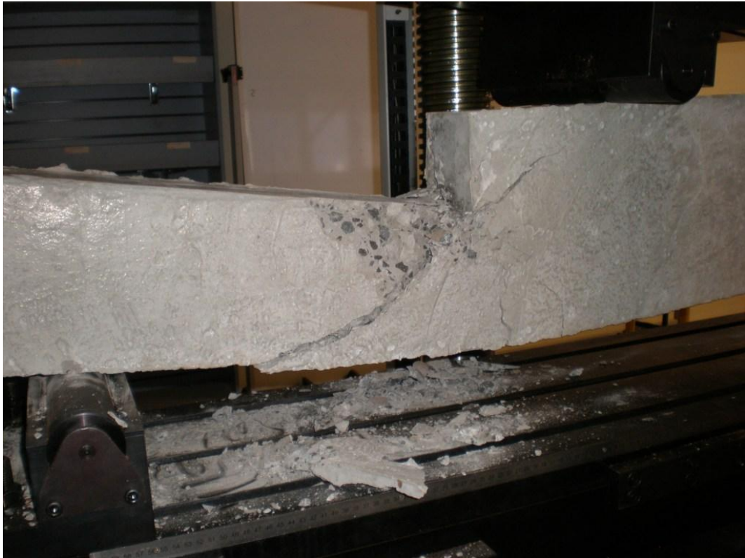
Photo 11 – Failure of conventional beam
