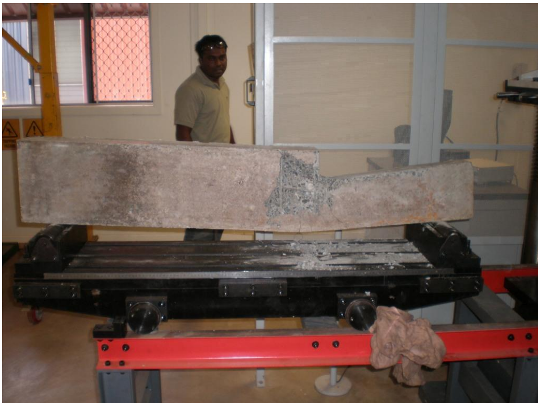
Photo 12 – Conventional beam at failure
