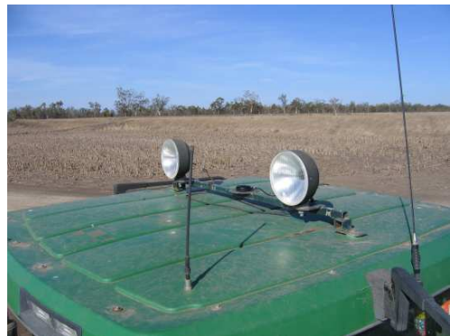
(d) Mobile GPS 18-5 receiver mounted on tractor
