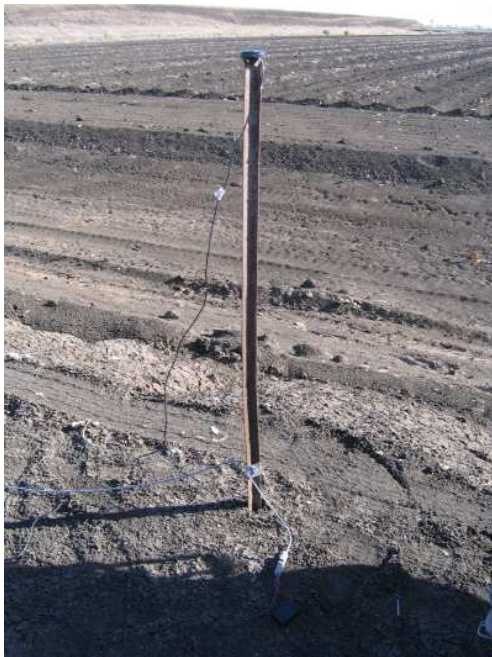
(c) Fixed GPS 18-5 receiver mounted on base station
