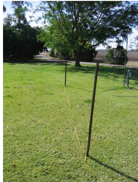
(b) Star pickets used to log receiver position over known distance
