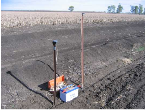
(a) Fixed GPS 35 receiver mounted on base station with Zigbee Transmitter (left)
