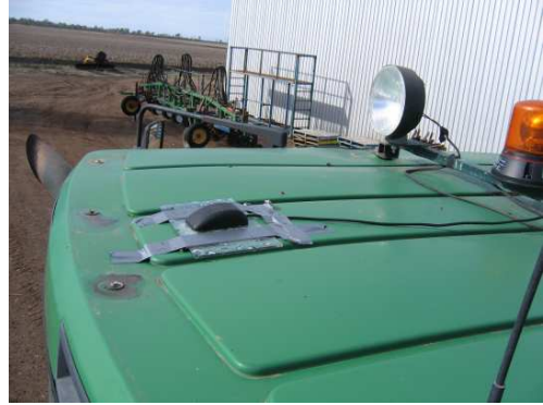
(b) Mobile GPS 35 receiver mounted on tractor
