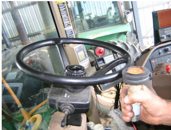
Figure 7.5: Motor configuration for testing hands-free guidance
