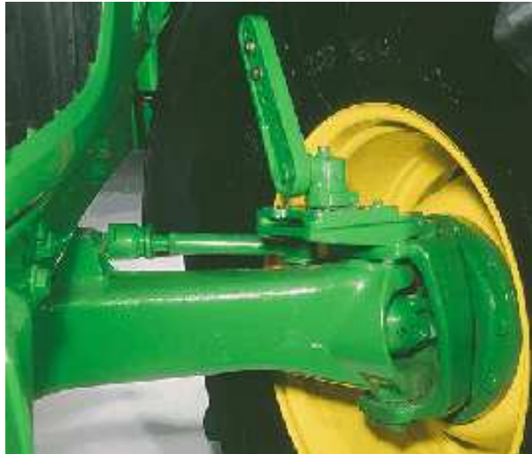
Figure 2.10: Example of hydraulic steering on farm tractor
