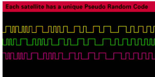
Figure 2.3: Pseudo Random Code Transmitted by GPS Satellite
