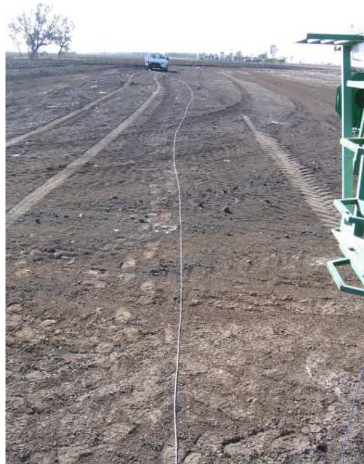
Figure 7.1: Transmission cable used to connect base station to machine
