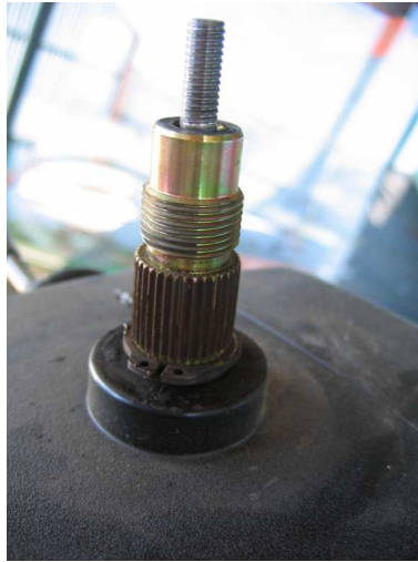
Figure 5.4: Steering column mounting point for gearbox
