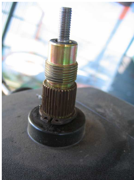
Figure 2.13: Steering column mounting point for gearbox
