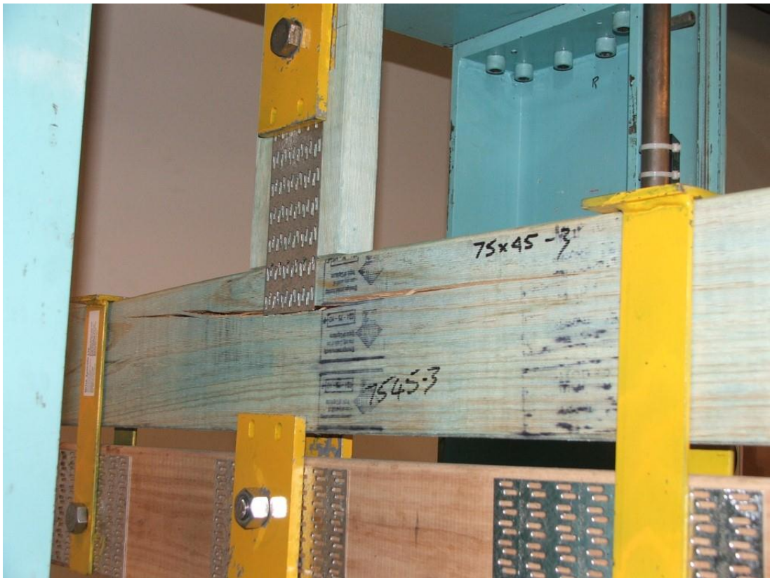
Figure 4.11 - Possible fracture restricted by over straps
