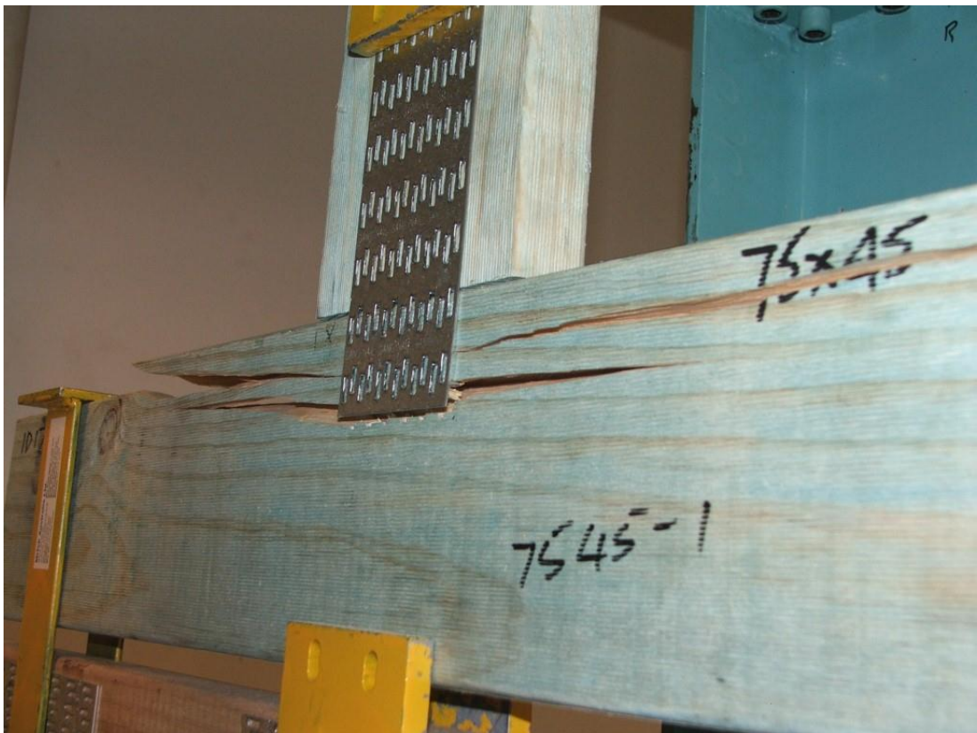
Figure 4.9 - Two noticeable fracture lines on front
