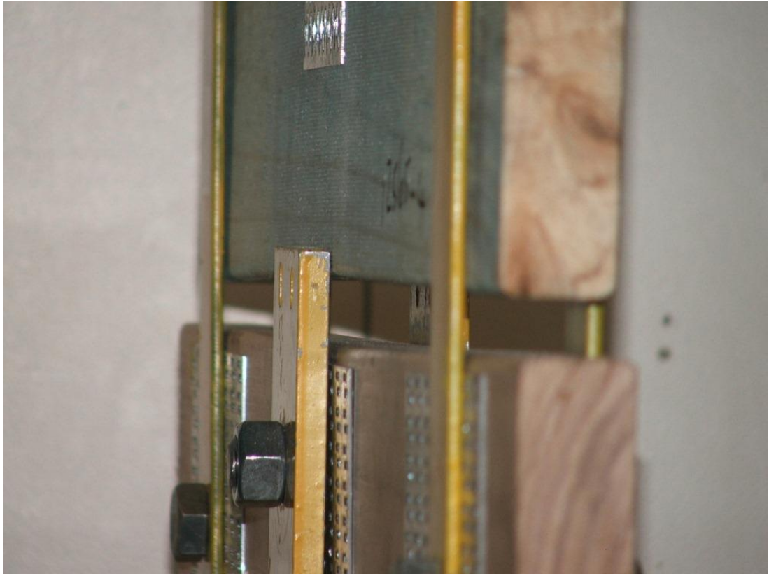
Figure 4.24- Noticeable deflection of both bending beam and sample
