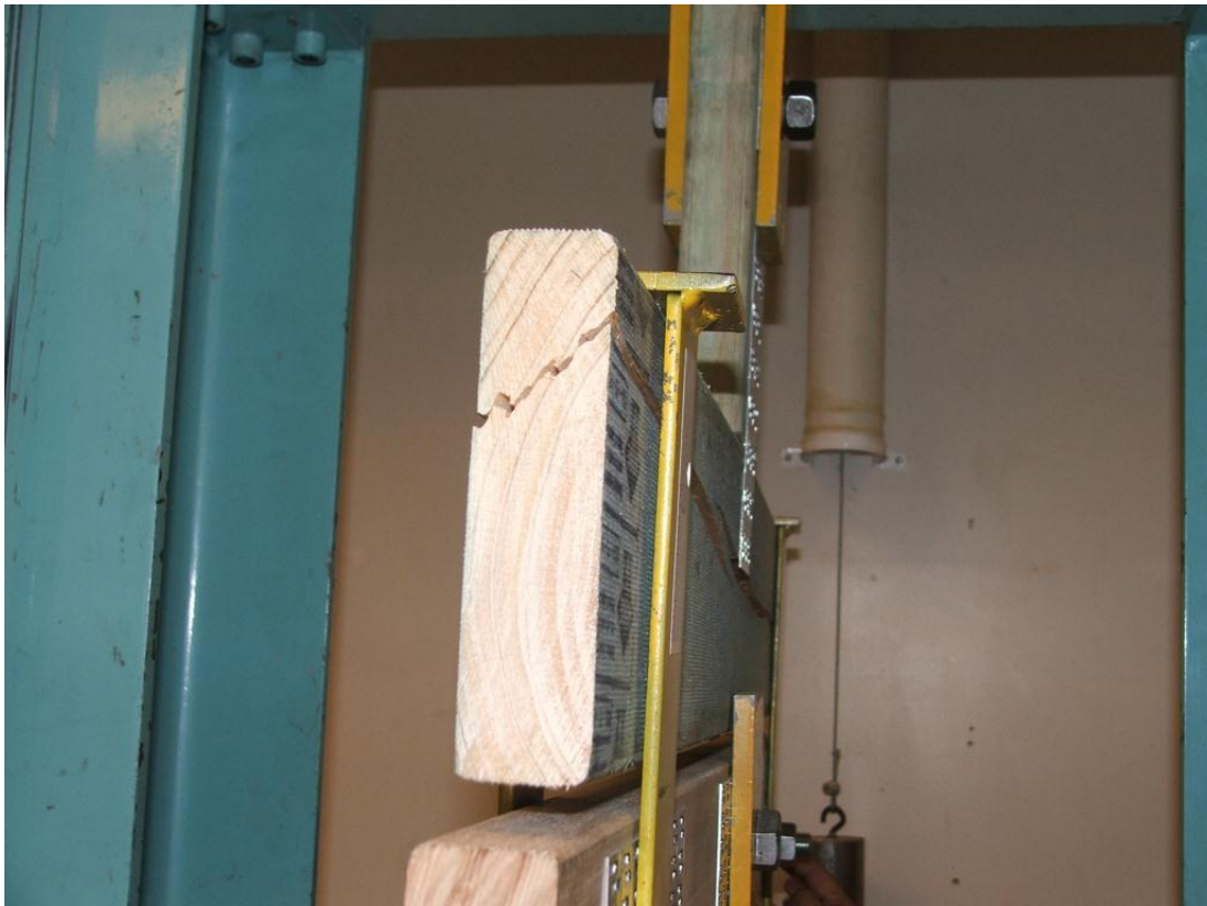
Figure 4.7 - Fracture follows grain in cross section
