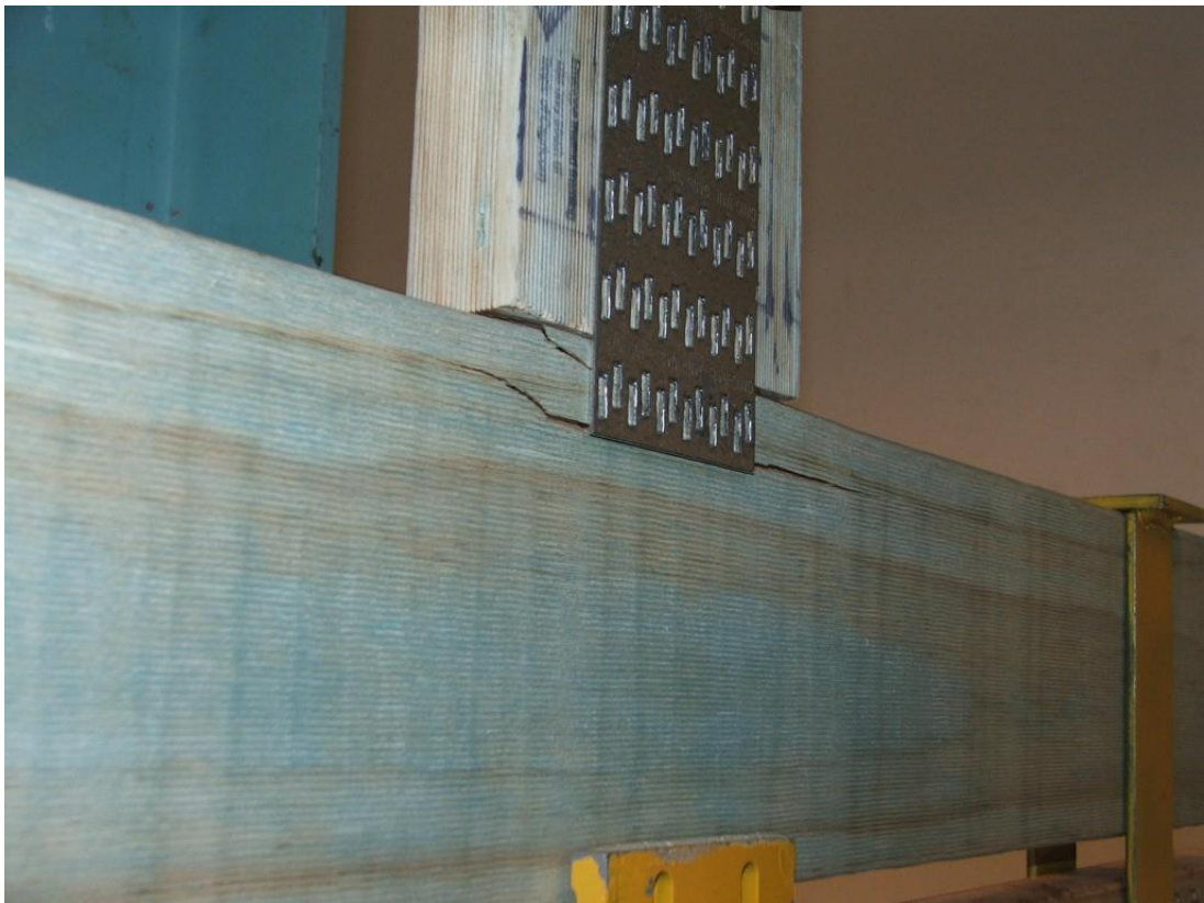
Figure 4.14 - Minor fracture along bottom row of teeth both top and bottom
