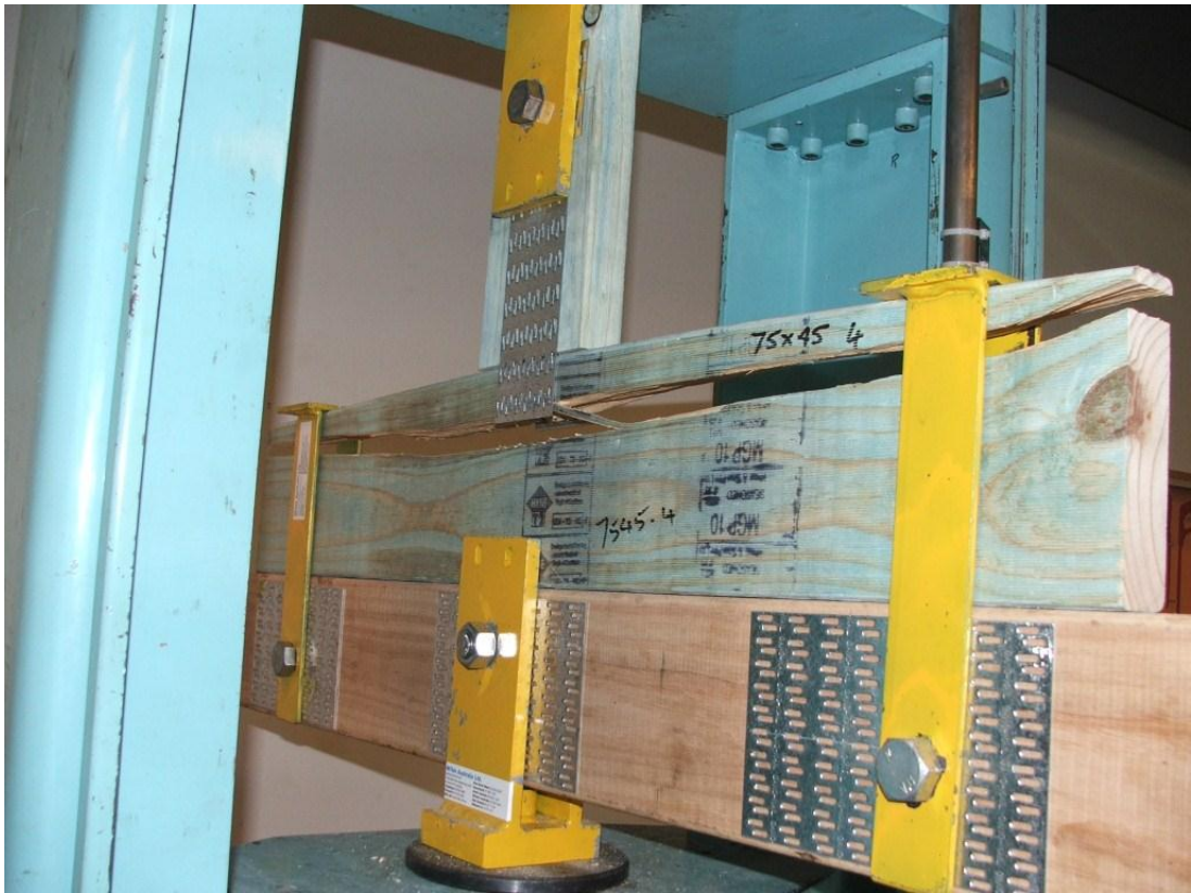
Figure 4.12 - Full fracture following grain around defects
