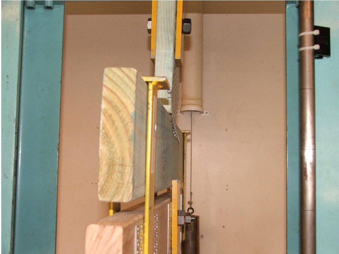
Figure 4.19 - Occurrence of substantial plate withdrawal
