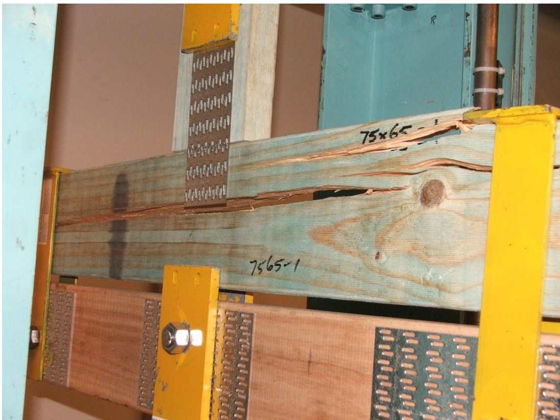
Figure 4.8 - Fractures following grain around knots and other defects
