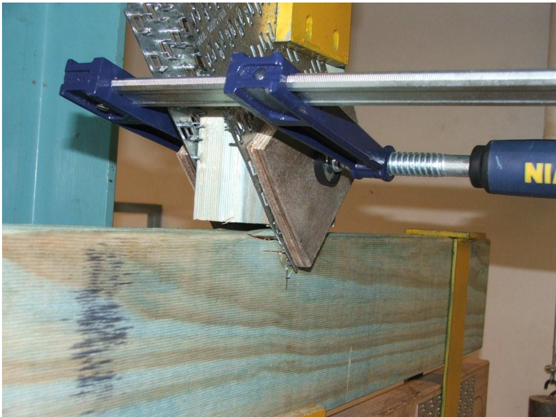
Figure 4.22 - Continued force after withdrawal and achieved failure, but not reliable values.
