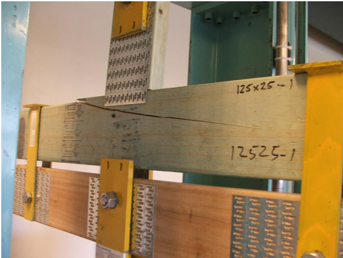
Figure 4.3 - Sloping failure along grain. End fibres remain intact
